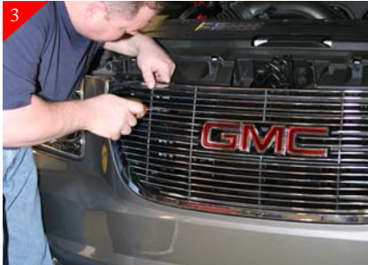
Simply tighten up the toggle bolts. To help start bolts it maybe necessary to pull out on the billet grille so that there is something for the bolt to tighten against. Another method is to use a second screwdriver to help hold the wing nut until it snugs up against the shell.
