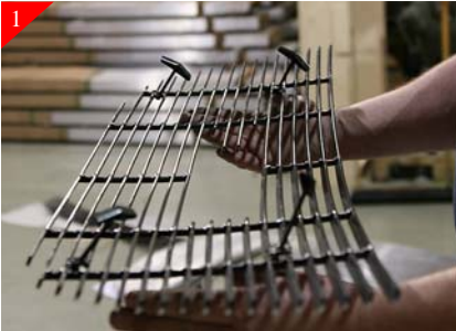
Place toggle bolts thru mounting tabs in billet grille as shown above.
