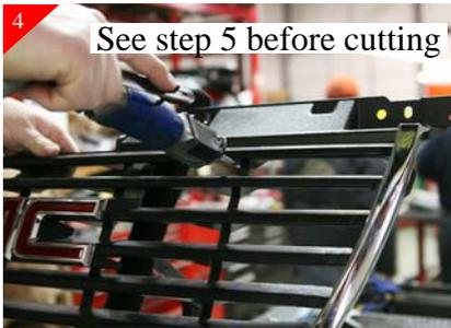
After removing center portion of stock grille shell lay on a protect work surface. Then using a hack saw, or air/power saw cut all the vertical and horizontal plastic bars. Make sure to leave enough material to do finish sanding.
