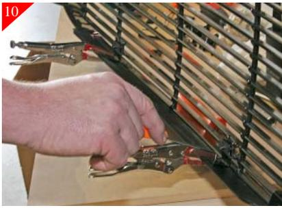
Place billet grille into stock shell and center. Then using a pair of vice grips clamp in place. Make sure to check alignment before marking. With the billet grille aligned using a scribe mark all the hole locations in brackets as shown above.
