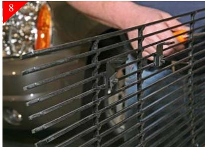
Using the supplied #8 x 5/8" Phil pan head screws attach the (4) Top brackets to billet grille as shown.
