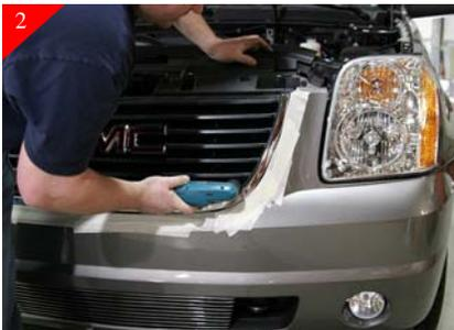
Locate and remove (4) 7mm bolts across top of core support and (6) 10mm bolts that surround hold the stock grille shell in place as shown above.
