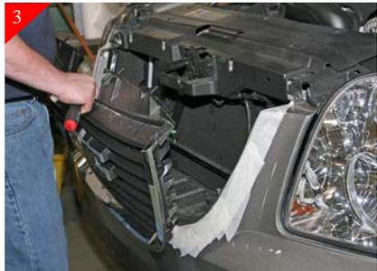
There are (8) clips total that hold the chrome or (center) portion of the stock grille shell to the painted portion of the front end. You will need to release these clips, do so by pushing the center of the clip to release.
