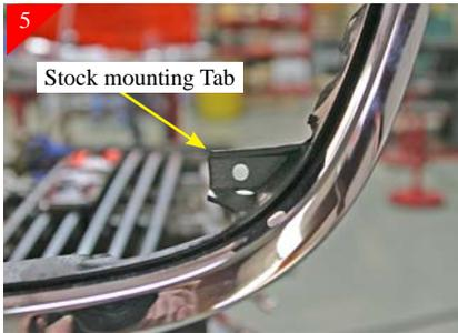
When removing the center, take note of the mounting tabs in the lower left and right sides of the shell. You will need to trim around these areas. These will attach the shell back the vehicle.
