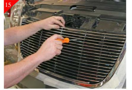
Next place the billet grille into stock shell and center. Then attach billet grille to the brackets using the supplied #8 x 5/8" Phil pan head screws as shown above. Remove the masking tape and the installation is complete.
