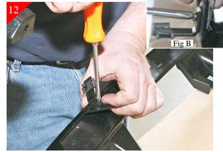
Remove the brackets from the billet grille. Then attach the brackets to the stock shell using the supplied U-clips and #8 x 5/8" Phil pan head screw. The U-clips go on the underside. (See fig. B to see the attach u-clips.)
