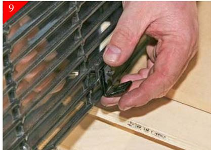
Using the supplied #8 x 5/8" Phil pan head screws attach the (2) Bottom brackets to billet grille as shown.
