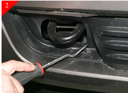
2 Then using a regular screwdriver or pry tool remove the rivets as shown above and repeat for the other side.
