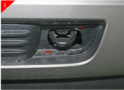
1 Locate the (2) plastic rivets in the tow hook area shown above in RED.
