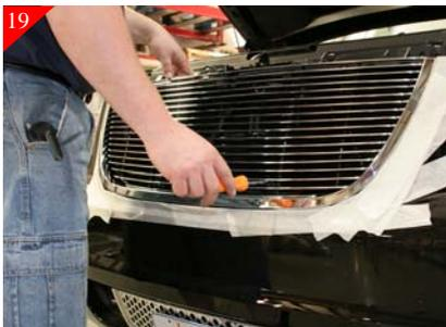
Next place the billet grille into stock shell and center. Then attach billet grille to the brackets using the supplied #8 x 5/8" Phil pan head screws as shown above. Remove the masking tape and the installation is complete.
