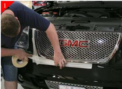
To protect you stock shell during the installation tape the painted portion surrounding the chrome on the front end of your vehicle using masking tape.
