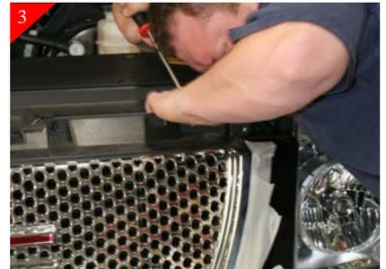
There are (8) clips total that hold the chrome or (center) portion of the stock grille shell to the painted portion of the front end. You will need to release these clips, do so by pushing the center of the clip to release. A long handled regular screwdriver may aid in the release of the clips.
