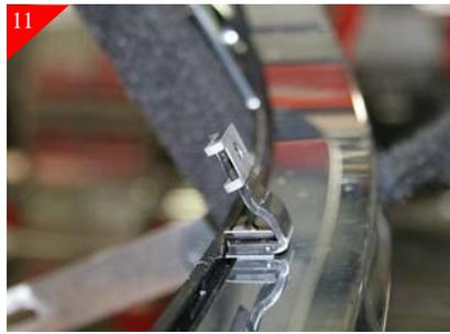
Attach bottom brackets to stock grille shell using the supplied #8 x 5/8" Phil pan head screws as shown above. Phillips screws come up from the bottom.
