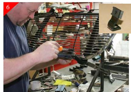
Place billet grille into opening and center. Next place supplied u-clips on Bottom brackets as shown above. Then attach brackets to billet grille using supplied #8 x 5/8" Phillips head screws as shown.
