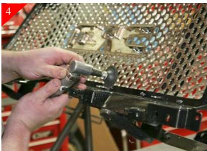
After removing center portion of stock grille shell lay on a protective work surface. Using a grinder, air sander, or dremmel grind all the plastic welds that hold center section in place as shown.
