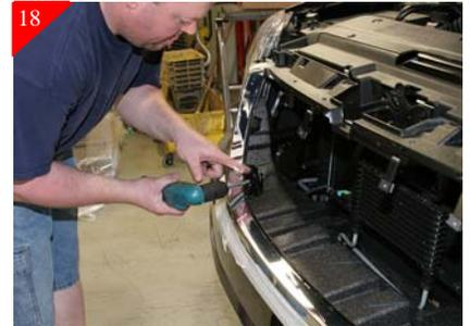
Place the stock shell back on vehicle by pushing the clips back in place and attach using the stock hardware (Ref step 1).
