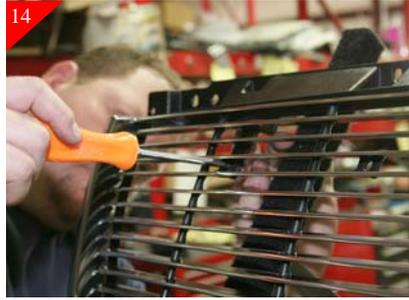
Using the supplied #8 x 5/8" Phil pan head screws attach the (4) Top brackets to billet grille as shown.
