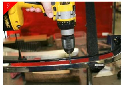
Remove the billet grille from stock shell. Also remove the bracket from the billet grille. Using a 3/16" drill bit, drill in the just marked locations.
