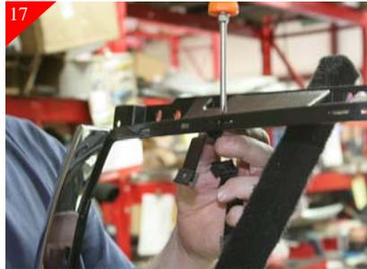
Remove the Top brackets from the billet grille. Place a u-clip on the short end of Top bracket then attach Top brackets to the stock shell using the supplied #8 x 5/8" Phil pan head screw as shown above.
