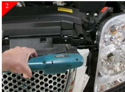
Locate and remove (4) 7mm bolts across top of core support and (6) 10mm bolts that surround and hold the stock grille shell in place as shown above.
