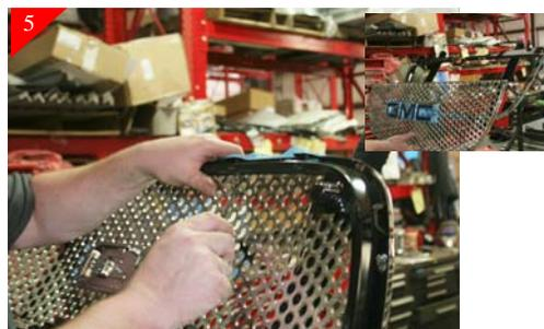
Remove the center chrome section, by using a regular screwdriver and pry out on all the plastic weld areas to release. Center section will be free at this point.
