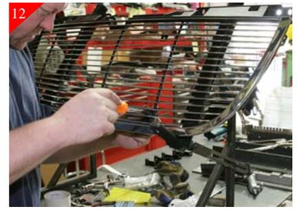
Place billet grille into opening and center. Attach bottom portion of the billet grille to the just placed brackets using the supplied #8 x 5/8" Phil pan head screws.
