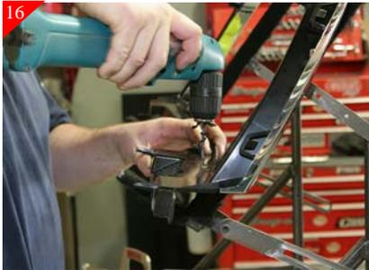
Remove the billet grille from opening. Using a 3/16" drill bit drill all the just marked areas as shown above. It may be easier to flip grille shell over during the drilling process as shown above.
