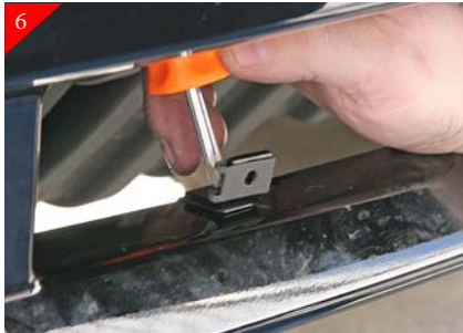
6 Place the supplied U-clips on the just drill holes as shown above. Remove brackets from the billet grille and attach the brackets to the just place U-clips as shown above. Note: You will may need to use a short Phillips screws driver to attach the bottom brackets. Repeat and attach the top brackets.
