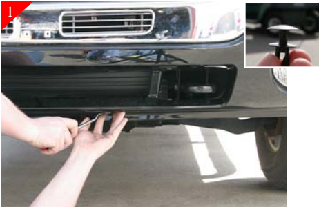
1 Your vehicle may or may not be equipped with Plastic bumper guard as shown above. If so you need to remove, do so by removing the (4) plastic push pull rivets.
