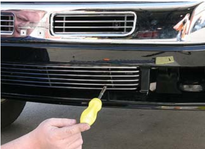
7 Attach billet grille to the just place brackets and tighten.
