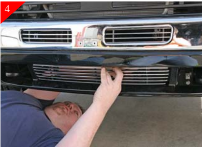
4 Place billet grille into opening and center. Reaching up from under the vehicle using a scribe mark the hole locations where they meet the vehicle as shown above.
