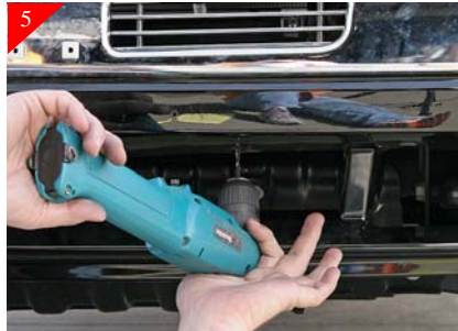
5 Drill a 3/16" hole in the just marked locations.
