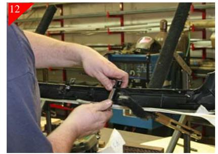
Attach the brackets to the stock grille shell using the supplied 1/4-20 x 3/4" bolts and 1/4-20 Nyloc nuts as shown above.
