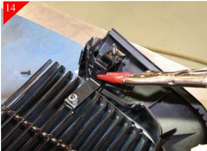
Attach the upper "L" brackets to billet grille and then using a pair of vice grips clamp in place as shown above. Then using a scribe mark the locations and then drill a 9/32" hole in each of the marked locations.
