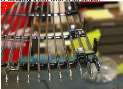
7 Attach brackets to billet grille using the supplied 1/4 - 20 x 3/4 bolts and 1/4 - 20 Nyloc nuts as shown above.
