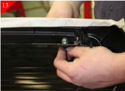
Place the billet grille back into opening and center. Then attach billet grille to the just attach brackets.
