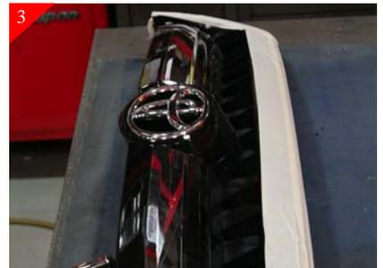
3 Tape the stock grille shell using masking tape to protect during install.
