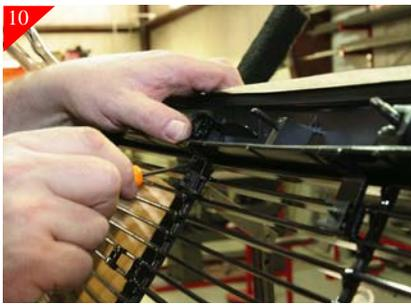
Using a scribe mark the location of the holes in brackets where they meet the stock shell.
