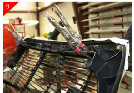
9 Align the brackets with the backside of the stock grille shell. Then using a pair of vice grips clamp in place.
