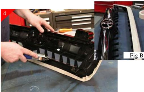
4 (Fig B) shows the completed cutting of the stock shell, you will be using the Top piece only. Cut the vertical fins that connect to the upper portion of stock shell that you will be keeping as shown above. Also go ahead and remove the stock hood release bracket, you will be re-installing a little latter in the install..
