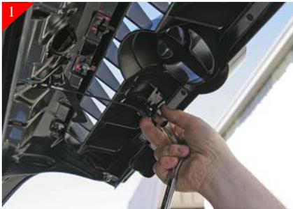
1 Open hood and remove (2) 10mm bolts that hold stock hood release.
