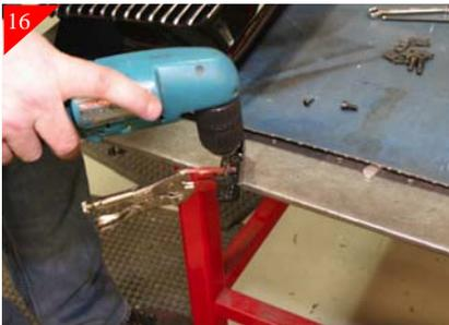
Drill a 9/32" hole in the stock hood release brackets to allow for the new bolts to pass thru. Make sure to clamp to a solid work surface before drilling.
