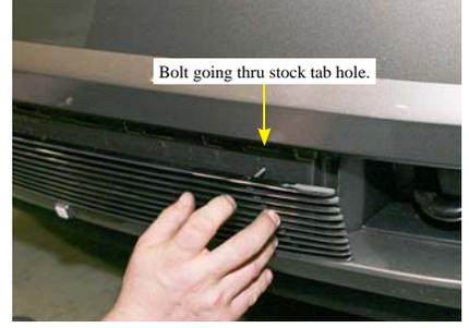
Now place billet grille into opening and center. There are slots in the bumper opening where the tabs on the black plastic bumper cover attached. This is where the bolts go thru. (Ref step 3).
