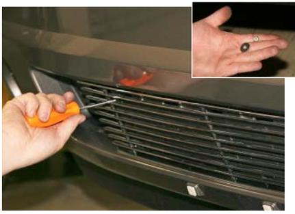
Attach the billet grille using the supplied Nyloc nut and washer.
