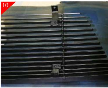
Next you will need to place the U-Clips on all of the long ends of the brackets. Attach brackets to the billet grille using the supplied #8 x 5/8" phil pan head screw. The long brackets will attach to the TOP of the billet grille. The SHORT brackets will attach to the bottom of the billet grille as shown above.
