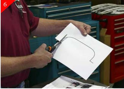
Shown above is the template to be used for the rest of the trimming process of the shell. The full scale template to be used is on the following page. You will need to cut out template as shown. Keep top portion.
