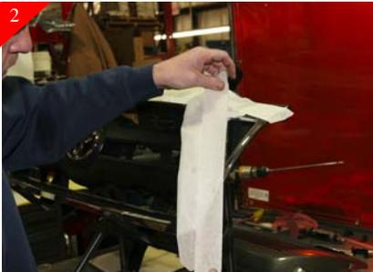
With grille shell removed using making tape, tape the front of the stock grille shell to protect during install.
