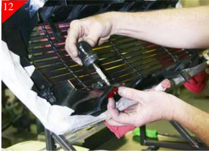
Then attach billet grille using the supplied #8 x 5/8" phil pan head screw and U-Clips as shown above. Take note that the U-Clip goes on the outside of the grille shell shown above in RED. Tighten all hardware. Then re-install grille back on vehicle.
