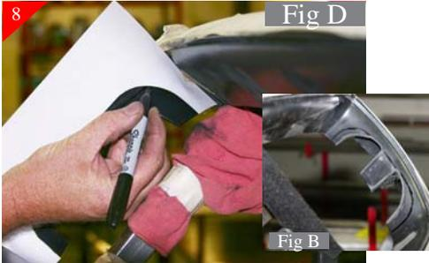
(Fig. A) Next using the template as a guide mark using a sharpie or scribe as shown above. (Fig B) shows the cut line to follow after marking.
