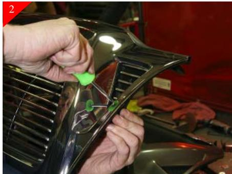
After drilling place the wing billet grilles back into opening and center. Then attach grilles by placing u-clips on the backside of the stock shell and attach with #8 x 5/8" Phillips pan head screws as shown. Tighten the bottom screws first and then the top screws.
