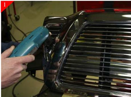
Place wing billet grilles into place and center. Then using a scribe mark the locations of the holes. Remove billet grilles and drill a 3/16" hole in each of the marked locations.
