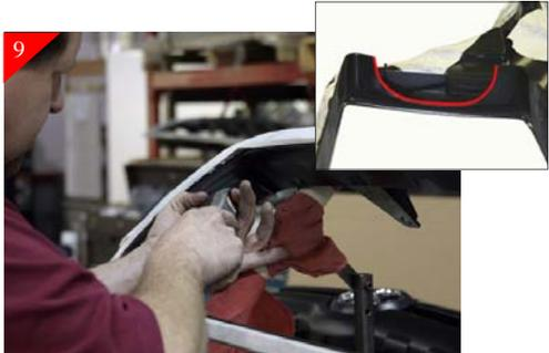
Cut along just marked line using a hack saw blade or cut off wheel.
