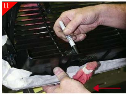
Place billet grille into opening and center. Using one hand as shown above make sure that the billet grille is flush with the face of grille shell. Then mark location of bracket against grille shell.
