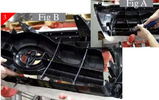
Next you will be removing the center section of the stock grille. Using a hack saw blade or cut off wheel remove as shown above (Fig A). Making sure to leave material for finish sanding. (Fig B) showing center section removed.
