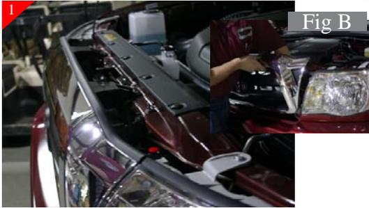
Remove the stock grille shell from vehicle by removing the 2 bolts along the top of the grille shell and then the bottom of the grille shell is held by 2 snap clips. There is also (2) plastic push pull rivets shown above in red. With the top 2 bolts removed lean the grille shell forward and reach behind and release (Fig. B)
