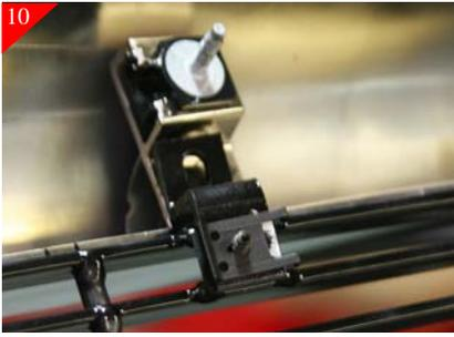
Attach Top brackets to billet grille using the supplied U-clips and #8 x 5/8" Phil pan head screws as shown above. Using a scribe mark the hole locations where it meet the stock shell. Drill just marked holes using a 3/16" drill bit.
