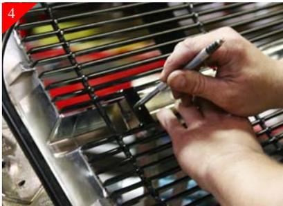
4 Place billet grille into opening and center. Next using a scribe mark the hole locations where the mounting bracket meets the stock grille shell as shown above. Repeat for the other center brackets.
