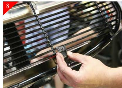
8 Attach the supplied Bottom brackets to the billet grille using the supplied U-clips and #8 x 5/8" Phil Pan head screws as shown above.
