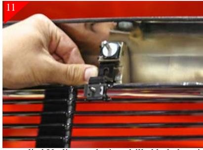
Place supplied U-clips on the just drilled hole locations. Now attach bracket to stock shell using supplied #8 x 5/8" Phil pan head screws.
