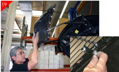
There are 6 studs on the shell. These 6 studs go through the hood. The "Z" brackets install on the 4 studs in the center of the shell. Now place the grille on the hood. Finger tighten nuts on the two outer studs to hold the grille in place. Now you are ready to install the 4 "Z" brackets to the Studs and finalize attachment of the grille to the hood. **Do not allow the hood to shut as possible damage could occur to painted bumper.**
