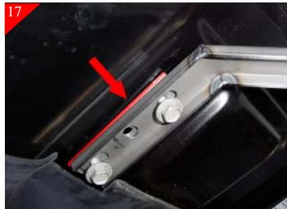
Place the flat "slotted" brackets between the "slotted Y" hood brackets and hood and re-install the (4) factory hood bolts. **Finger tighten only.** The brackets have slotted holes for alignment adjustments later.
