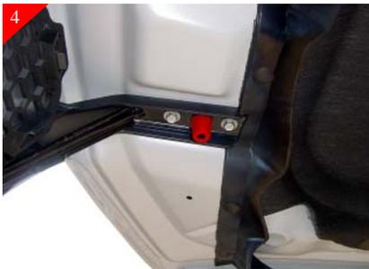
Remove the two rubber stops on the brackets and **SAVE** them. They will be reinstalled.
