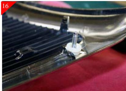
Now place the plastic washers on the studs located on the outer side of the grille. There are four total. Carriage Works suggests applying some silicone on the plastic washer so it stays in place during installation
