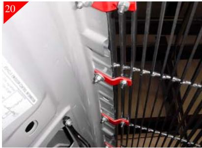
Using a slight upward pressure on the bottom of the grille attach the four supplied "Z" brackets to the billet grille as shown using the factory nuts and the supplied 1/4"-20 bolts and nuts as shown. These brackets will be tight as they are used to hold the grille and shell in the correct final position. Tighten all "Z" bracket nuts and bolts. Make sure that the grille shell forms to the face of the hood.
