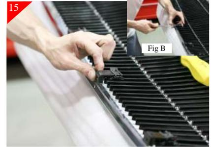
After drilling place supplied U-clips on all the lower brackets as shown above. Then attach brackets to stock shell by using the supplied #8 x 5/8" Phillips head screws as shown above (Fig. B). Screw by hand with a screwdriver so they will not strip the thread. If done correctly the heads will sit nice and flush. You may need to file any burrs off after tightening.
