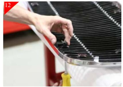
Place supplied U-clips on long end of the (4) lower brackets and attach to billet grille using the supplied #8 x 5/8" Phillips head screws.
