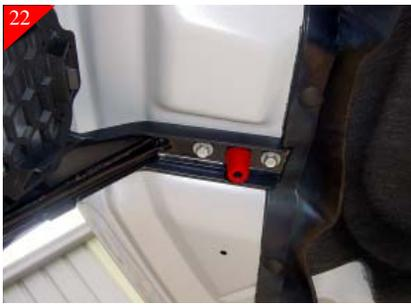
**The rubber bumpers previously removed from the grille brackets must now be re-installed. Failure to reinstall may cause damage to the Vehicle.**
