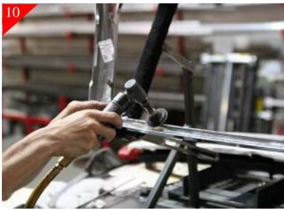
With all the tabs removed sand all cut areas smooth using a sanding block or air sander.
