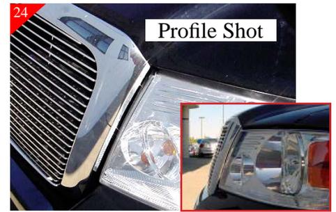
Adjust the bottom of the grille for proper alignment using the headlight lens as a guide for spacing by loosening the (2) - (10mm) bolts on the hood and the (6) Bolts holding the grille to the "Slotted Y" hood brackets. Once adjusted properly tighten all bolts and nuts.
