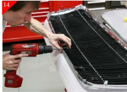
Using a 3/16" drill bit drill all the just marked locations.
