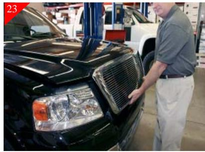
**Carefully** lower the hood and check the alignment of the grille with the headlights. **Do not allow full weight of the hood or use force to close the hood as damage may occur to the bumper cover.**
