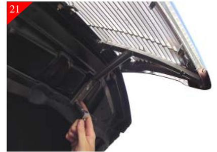
Next, using the remaining 1/4"-20 nuts and bolts, attach the grille to the vertical bars of the hood brackets. Then tighten all remaining "Slotted Y" brackets, bolts, nuts, and hood bolts.
