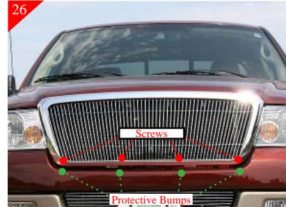
Next place the clear self adhesive protective bump stops as shown above. Place them on the bumper mask directly below the screws on the vertical rods. Again check for alignment. Installation is complete.
