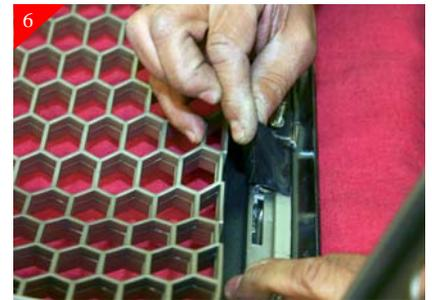
Now separate the outer shell from the honeycomb factory grille, but first you need to remove the fiber tape covering the clips.
