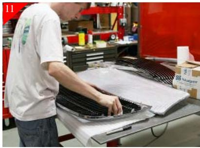
With all of the tabs removed and sanded, lay grille shell face down on a protected work surface. Then insert the billet grille and center as shown above.
