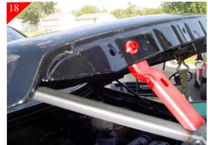
Next, attach the supplied "slotted Y" hood brackets with flat side of the bracket on the inside of the hood using the 1/4"-20 x 3/4 Hex screw, flat washer, and safety nut. **Again Finger Tighten Only.** Note: Passenger side bracket shown above with Red.
