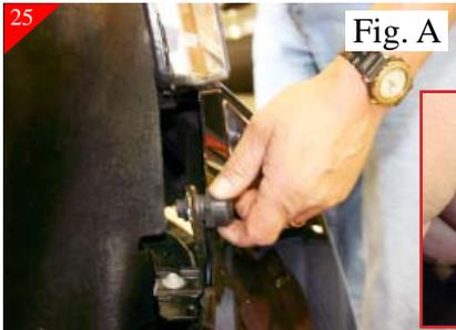
**(Fig. A)** Then adjust the rubber bump stops at the bottom of the grille so that the grille barely touches when hood is closed. **(Fig. B)** There should be 1/4" between top of bumper cover and bottom of screw head.
