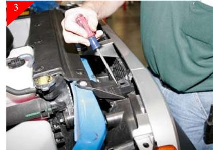
Next locate (2) clips shown above and release using a regular screwdriver to aid in the release. With the top clips released now locate the (3) clips along bottom of stock grille shell and release using the same method as the top.
