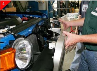
Stock shell will be free at this point. Remove and lay stock shell face down on a protected work surface.
