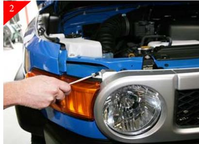
Locate the (2) plastic rivets one on each end of the stock shell shown above and remove.
