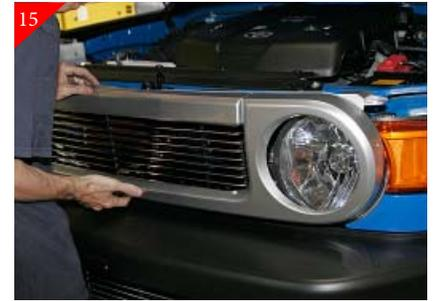
15 Re-attach stock shell to vehicle. Install complete.
