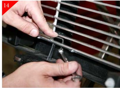
14 After drilling place billet grille back into opening and center. Attach billet grille using the supplied 10-32 x 1/2 bolts and 10-32 Nyloc nuts. Place supplied bolts thru mounting tabs in billet grille and thru the just drilled locations and attach using the nuts on the underside of the stock shell as shown.
