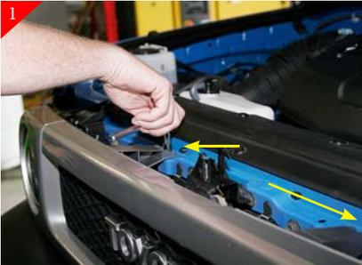
Remove (2) 10mm bolts that hold stock grille shell in place.
