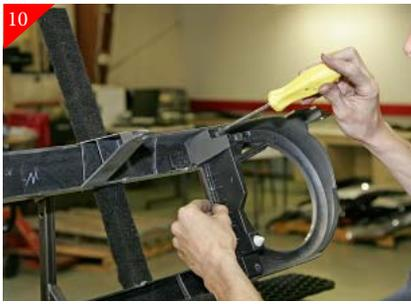
10 After sanding attach both plastic pieces back to stock shell using stock hardware as shown. (Reference step 5).
