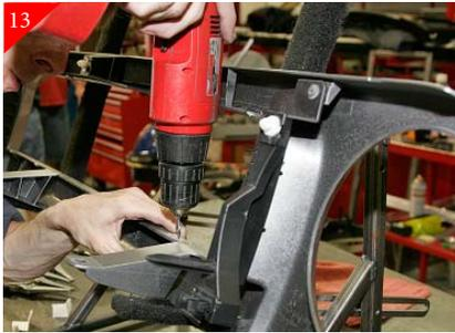
13 Drill all marked locations using a 3/16" drill bit as shown above.
