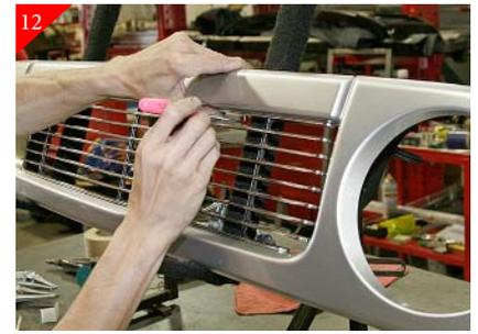
12 After aligning billet grille mark the (6) mounting locations using a 90° scribe as shown above. After marking remove billet grille from opening.
