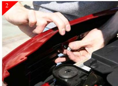
Reaching thru the top, remove the (3) metal nuts across the top and the sides as shown above. Next reaching thru the bottom of the grille release the (4) snap in tabs.
