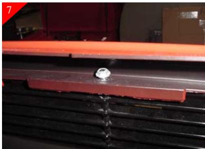
Now attach the 3 sheet metal nuts to the rods on the top of the grille shell and tighten, then re-install core support cover.
