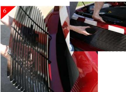
Place the bottom rods into the just drilled holes and gently pull up on the top crossbar of the grille shell and insert the top rods into the holes as shown above.
