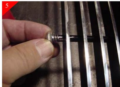
Using the supplied sheet metal nuts, pre-install on the top (3) rods and then remove them. This will make it easier to install during the final installation.
