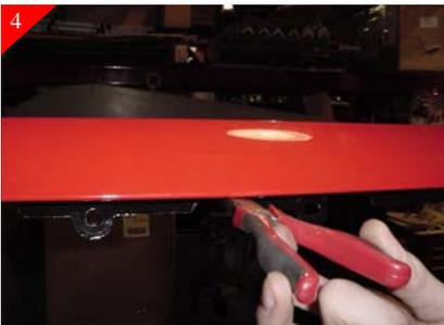
Using a pair of cutters, remove the 2 sets of alignment ribs on the top of the grille opening as shown.
