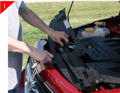
Remove the core support cover by removing all plastic rivets and screws.
