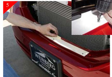
Next, using the supplied drill templates for the top and bottom, fold the templates on the dotted lines and center them on the tab on the top of the grille and in the slotted opening on the bottom of the grille. Make sure the back of the template is tight against the back of the grille opening and mark the location of the holes using the center-lines provided. Drill 3 places on top and bottom using a 9/32" drill.
