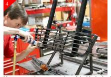
Next remove the center portion of the black plastic backing. Do so by using a air saw, cut-off wheel, or hack saw and cut all the vertical and horizontal plastic point where it meets the outer ring.
