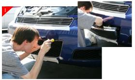
Start by removing the stock shell from bumper opening. Do so by releasing the clips holding in place, it maybe necessary to use a regular screwdriver in aiding in the release of the clips.
