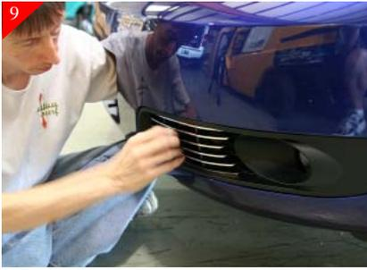
Place billet grille into opening and center. Next place the supplied toggle bolt thru mounting tab in billet grille. Reaching thru the center opening thread the "wing" portion of the toggle onto the bolt as shown above, there are 2 toggles per side.
