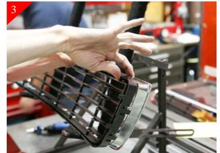
Remove the black plastic backing from chrome shell by un-clipping as shown above.
