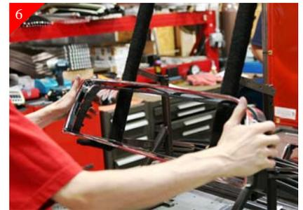
Re-attach the chrome ring and the black plastic backing together by snapping back in place.
