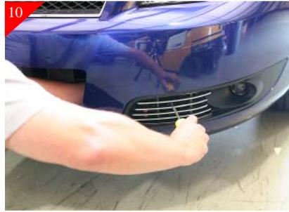
Using a Phillips screws driver tighten all the toggle bolts without over tightening. Over tightening may cause the stock honeycomb to crack. Please continue on with the install for the center portion of the billet grille steps 3-8 .
