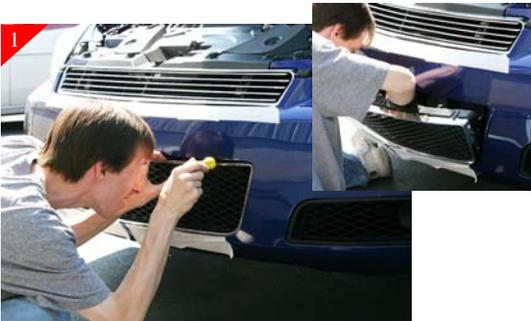
Start by removing the stock shell from bumper opening. Do so by releasing the clips holding in place, it maybe necessary to use a regular screwdriver in aiding in the release of the clips.
