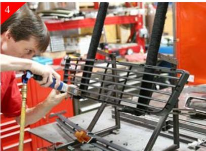
Next remove the center portion of the black plastic backing. Do so by using a air saw, cut-off wheel, or hack saw and cut all the vertical and horizontal plastic point where it meets the outer ring.
