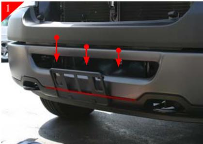
Remove the (5) 8mm bolts by reaching thru the front opening of vehicle. Area of bolts to be removed shown above in RED.
