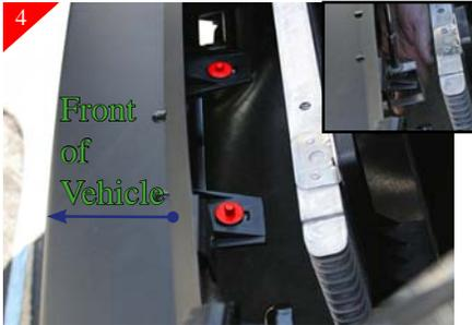
Next you will be attaching the top bracket to the factory 8mm bolts shown above. (Please Ref next step for diagram of attachment of brackets). Next locate the factory 8mm bolts on lower valance and remove, then attach the bottom bracket to these factory bolts. (Please Ref next step for diagram of attachment of brackets).
