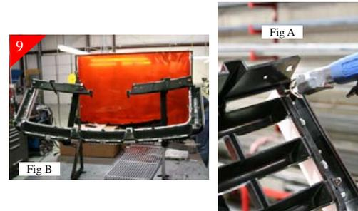
(Fig A.) shows cutting of the horizontal attachment points. (Fig B.) shows after cutting all attachment points and center removed.
