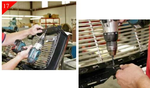
17 Drill all the just marked hole locations using a 17/64" drill bit.
