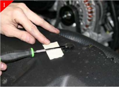
Remove the (4) plastic push pull rivets from along top of core support.
