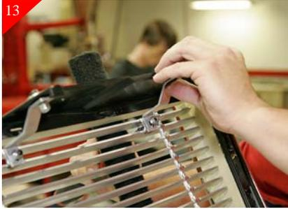
13 Now loosely attach the remaining (2) upper brackets to billet grille using the supplied 1/4-20 x 1" bolts & 1/4" Flat washers and 1/4-20 Nyloc nuts. The washer go on the head side of the bolt or on top of plastic.
