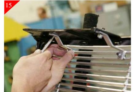
15 Repeat for other side--Using a scribe mark the mounting location where is meets the top of the shell as shown above.
