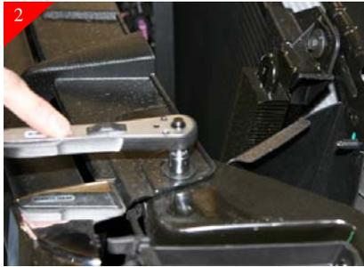
Remove the (4) 10mm nuts from top of stock grille shell.
