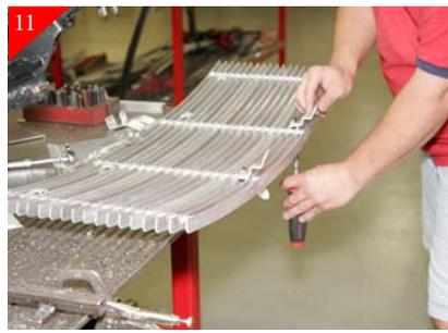
11 loosely attach the (2) bottom brackets using the supplied 1/4-20 x 1" Bolt and 1/4-20 Nyloc nuts shown above.
