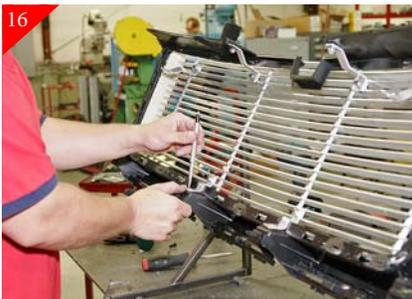
16 Using a scribe mark the mounting location where is meets the back of the shell as shown above. Make sure that the bottom brackets are firmly butted up against the black plastic shell before marking. Repeat for the remaining bottom bracket.
