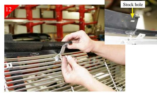
12 Loosely attach (2) upper brackets to the 2 inner mounting tabs in billet grille using the supplied 1/4-20 x 1" bolts and 1/4-20 Nyloc nuts. Now attach brackets to top of shell using the stock hole as shown above (Fig B), and also using the stock bolts. This will help hold billet grille in place while marking and drilling remaining mounting locations.
