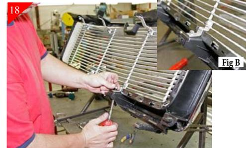
18 After drilling attach brackets using the supplied 1/4-20 x 1" bolts and 1/4-20 Nyloc nuts. Make sure the bottom brackets are butted against the black plastic (Fig B).
