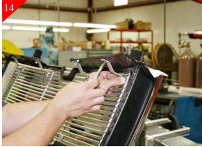
14 Using a scribe mark the mounting location where is meets the top of the shell as shown above.
