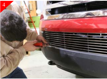
Rotate brackets around so that they catch or hook the stock plastic in bumper opening. Also use of an additional screwdriver to aid in the rotation of the brackets may be used.
