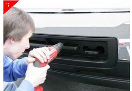
Using a 17/64" drill bit, drill in the just marked locations as shown above.
