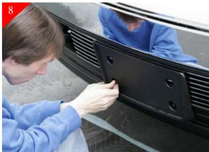
Attach license frame holder using the supplied 1/4-20 x 1" and small washers on the head side of bolts and large washer and 1/4-20 Nyloc nuts on backside as shown.
