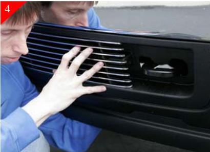
Place billet grille into opening and center. Place supplied 1/4-20 x 2/12" bolts into mounting tab and reaching behind bumper place the supplied washer and 1/4-20 Nyloc nuts and tighten. Being careful to not over tighten.
