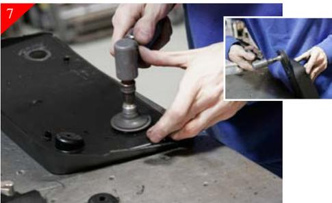
Using an air sander or sanding block sand all cut areas smooth as shown.
