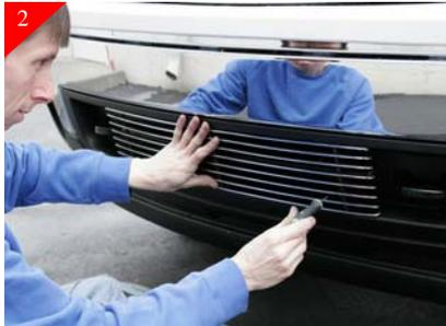
Place billet grille into opening and center. Using a scribe mark the hole location for the mounting tabs as shown above.
