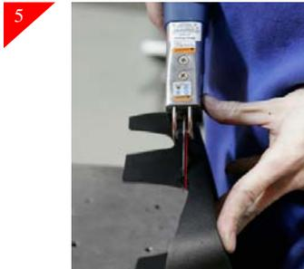
If your state requires you to have a front license plate please continue with install. Using the scribe line created in step 1 shown above in red. Using an air saw or other cutting tool cut along scribe line and remove that portion of the license frame holder.
