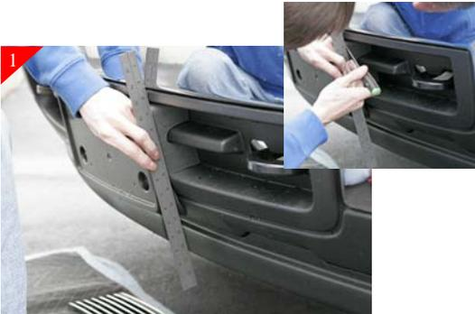
Start by using a straight edge as shown above. Using a scribe mark as shown above using the straight edge as a guide repeat for remaining side. You will be using this cut line later in the install to allow re-attachment of the license frame. If your state doesn't require a front license frame you can skip cutting the license frame.
