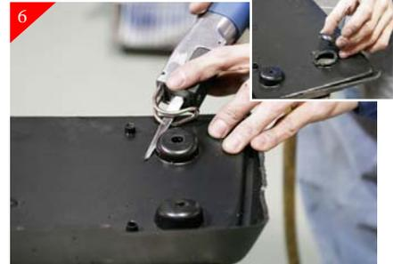
Turn license frame holder over face down. Remove the top mounting holes using an air saw or other cutting tool as shown above.
