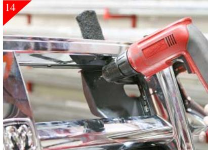
Remove the brackets from billet grille then remove billet grille from opening. Then using a 3/16" drill bit, drill all the just mark locations. When drilling holes for the center attachment be careful not to drill thru the chrome portion of the stock shell.
