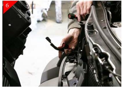
Remove The connections from the headlights (3) per light. The stock shell will be free at this point.
