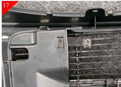
To Attach the Upper bracket locate the hole you drilled and place a supplied U-clip on the backside of plastic and attach by screwing to the U-clip as shown above. Install is complete. Center stock shell on vehicle and snap shell back in place and remember to attach all headlight connections. (Ref. steps 1-6).
