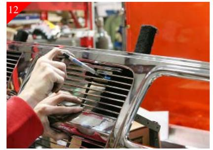
Mark The hole location for the Upper bracket using a scribe as shown.
