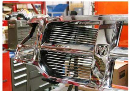
Insert the billet grille from the backside as shown above.
