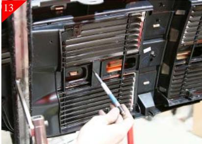
Again check the alignment of the billet grille. Then using a scribe mark the hole location as shown above.
