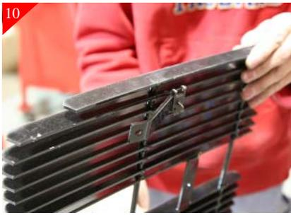
**Note:** Photo was taken while billet grille was not in stock shell to better show the attached bracket. Place supplied U-clip on Upper bracket as shown above. Then attach the bracket to billet grille using the supplied #8 x 5/8" Phillips head screw
