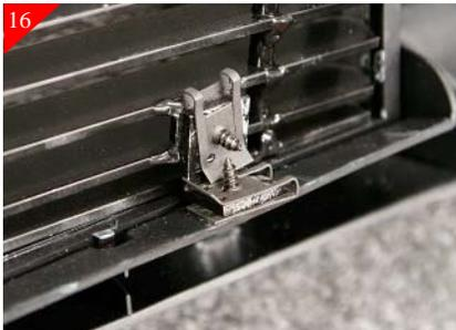
The bottom brackets attach using the supplied #8 x 5/8" Phillips head screws and U-clips as shown above.
