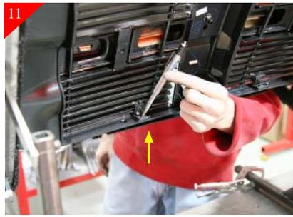
Place supplied U-clips on bottom bracket, then attach bracket to billet grille using the supplied #8 x 5/8" Phillips head screw as shown above. Check alignment of the billet grille and using a scribe mark the location of the hole in the bracket where it meets the stock shell as shown above.
