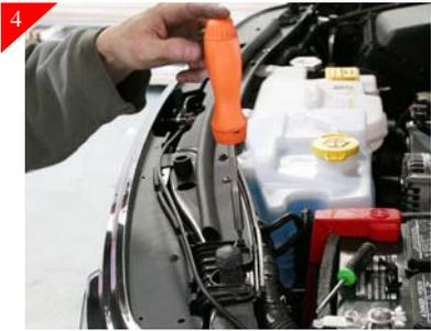
Remove (2) torx #25 screws per side holding headlights in place.
