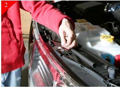
Next Release the hood release cable from the cable guides.
