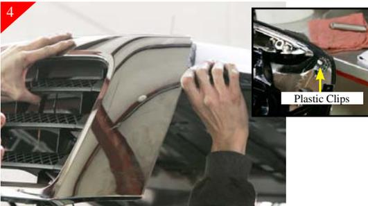
Next there are (2) plastic snap in clips one per side of stock grille shell. You need to pull out on the upper corners of the stock shell to break these clips. These clips serve only as a manufacturing aid. They don't have any structure of supporting functions. Also they are difficult to see but they are there. Grille shell will be free at this point.
