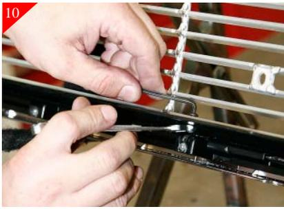
Place billet grille back into opening and center. Attach billet grille using the supplied 10-32 x 1/2" bolts and the 10-32 nyloc nuts.
