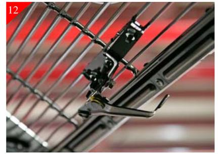
Now using the stock bracket from step 1, attach to the just placed bracket in step 11 using the supplied 10/32 x 5/8" and 10/32 Nyloc nuts.
