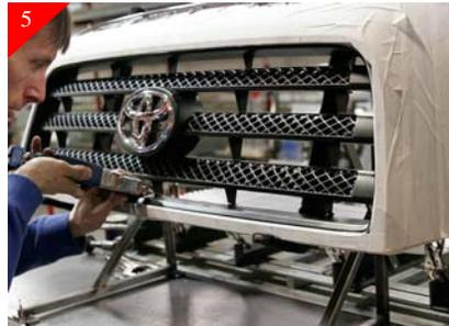
Using an air saw or other cutting devise. Remove the center portion of the stock grille shell by cutting all the horizontal and vertical attachment points. Make sure and leave material for finish sanding. See step 6 for cutting the vertical attachment point.
