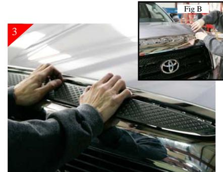
Remove the plastic rock guard from top of stock shell. Do so by unclipping at one end and working to the other. Then remove (5) 10mm bolts from under the plastic guard across top of stock shell as shown above (Fig B).
