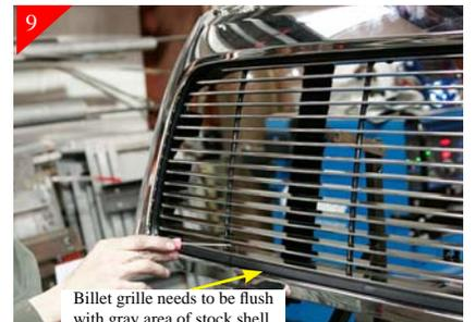
Place billet grille into opening and center. Make sure billet grille is flush top and bottom before marking. Using the billet grille as a guide, mark the hole location using a sharpie or scribe (4) on top (4) on bottom. After marking remove billet grille and Drill just marked location using a 7/32" drill bit.
