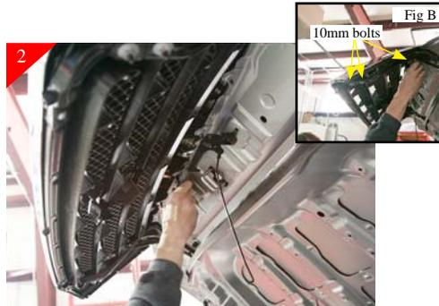
Remove (4) 10mm bolts located along top of stock grille shell as shown above. Locate and remove (3) 10mm bolts per side of stock grille shell shown in (Fig B).
