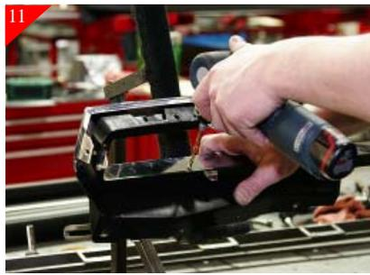
Next you will be drilling the top mounting hole locations. Turn stock grille shell over or face down then drill using a 3/16" drill bit. Flex or twist as in the previous step in order to reach and drill mounting holes as shown above. After drilling all mounting holes for the top portion re-install by clipping back in place.
