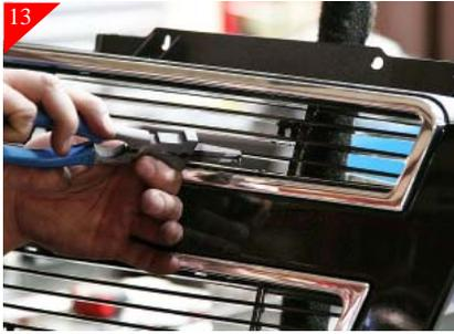
Place billet grilles into opening and center. Attach billet grille by using the supplied 10-32 x 5/8" bolts and 10-32 nyloc nuts. Replace the stock bolts that hold top portion of stock grille shell that were removed in step 8.
