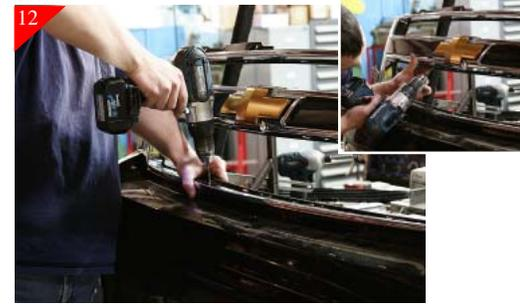
Move to the bottom portion of stock shell and drill the already marked locations using a 3/16" drill bit.
