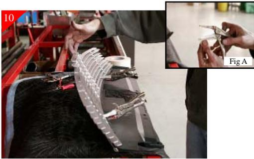
Tape a pair of vice grips using masking tape to protect during the clamping process (Fig A). Align the billet grille with the top portion of the stock shell. Then use the vice grips to clamp one end and then align and clamp the other end in place. Adjust as necessary to get the correct alignment.
