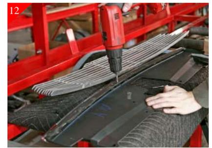
Drill the just marked hole locations using a 3/16" drill bit as shown above.
