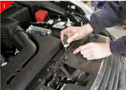
Open hood and remove (4) rivets shown above in red.
