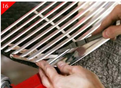
Align billet grille with the bottom portion of stock shell. Again using a pair of taped vice grips clamp in place. Using the supplied 10-32 x 5/8" bolts, place bolts in just drilled locations and secure with the supplied 10-32 nyloc nuts.
