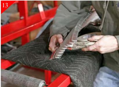
Next you will marking the hole locations for the bottom portion of shell. Following the same procedure as in step 10 for marking the top. Use a pair of taped vise grips and clamp one end of the billet grille and shell together, align and clamp the other end. Adjust as necessary to get the correct alignment.
