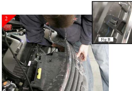
Locate the clips along bottom of stock grille shell. Release clips by lifting up and pulling outward on the shell. (Fig B) shows close up of the clips along bottom of shell. Grille shell will be free at this point.
