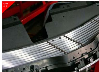
Following the same procedure as in step 16, align the billet grille with the top portion of the stock shell. Using vise grips to clamp in place. Using the supplied 10-32 x 5/8" bolts, place bolts in just drilled locations and secure with the supplied 10-32 nyloc nuts.
