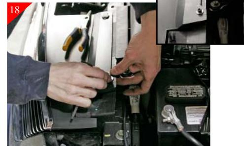
Next you will be attaching grille back to vehicle. (Ref steps 1 & 2) Place shell on vehicle and snap into place. Replace the factory rivets except for the outer (2) rivets in these locations you will fastening using the supplied 1/4-20 x 5/8" bolts and 1/4-20 Nyloc nuts with the washer going on the Top side of plastic as shown above. These bolts will allow for any adjustments that you may need to make. After adjusting tighten the (2) outer bolts.
