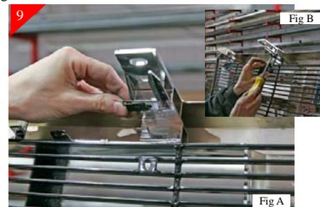
Place the supplied U-clips on the just drilled mounting locations as shown above (Fig A). Attach brackets to U-clips using the supplied #8 x 5/8" phillips head screws (Fig B). Place stock shell back on vehicle (Reference steps 1 & 2).
