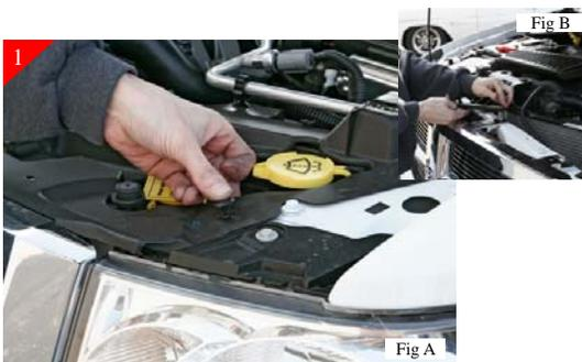
Start by remove the plastic core support cover. Do so by removing the (6) plastic push pull rivets from across top of cover (Fig A). Then locate and remove the (4) 13mm bolts located across top of stock shell shown above (fig B).
