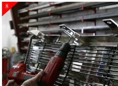
After marking hole locations, loosen bracket and swing out of the way for drilling. Drill the just marked locations using a 17/64" drill bit.
