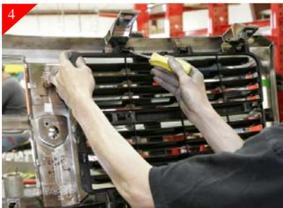
Lay stock grille shell face down and remove the black plastic backing by unclipping all attachment point.
