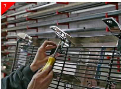
Attach billet grille to the just drill hole locations using the supplied 1/4-20 x 1 1/4" black bolts and 1/4-20 Nyloc nuts. Place the nut on the underside of the just drilled holes and attach using the supplied bolt. Now attach the supplied brackets to the top mounting tabs in billet grille using the supplied U-clips and #8 x 5/8" screws. After attaching brackets using a scribe and mark the mounting hole locations as shown above.
