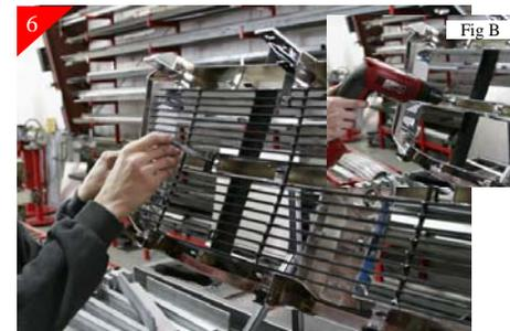
Move stock shell to protective works surface. Using masking tape, tape the face of the grille shell to protect during the installation.
