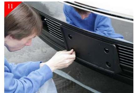
Attach license frame holder using the supplied 1/4-20 x 3/4" and washer on the head side of bolts and washer and 1/4-20 Nyloc nuts on backside as shown.
