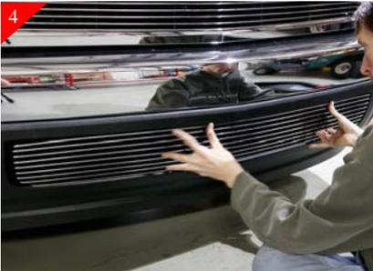
Place the supplied 10-24 x 2" bolts in the mounting tabs in billet grille. Now place the supplied spacers on the backside of the billet grille, slide the spacers on 10-24 x 2" bolts. Place billet grille back in opening and align with drilled holes. Push the 10-24 bolts thru the already drilled holes. Reaching from under front end place supplied washers on bolts and tighten using 10-24 Nyloc nuts.
