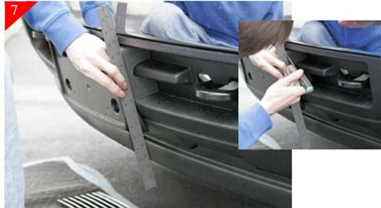
If your state requires you to have a front license plate continue with install. Start by using a straight edge as shown above. Using a scribe mark as shown above using the straight edge as a guide repeat for remaining side. You will be using this cut line later in the install to allow re-attachment of the license frame. If your state doesn't require a front license frame you can skip cutting the license frame.
