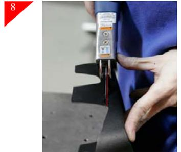
Using the scribe line created in step 7 shown above in red. Using a air saw or other cutting tool cut along scribe line and remove that portion of the license frame holder.
