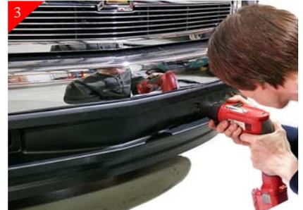
Drill just marked locations using a 1/4" drill bit.
