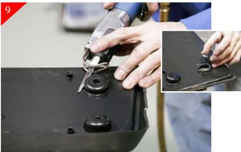
Turn license frame holder over face down. Remove the top mounting holes using a air saw or other cutting tool as shown above.
