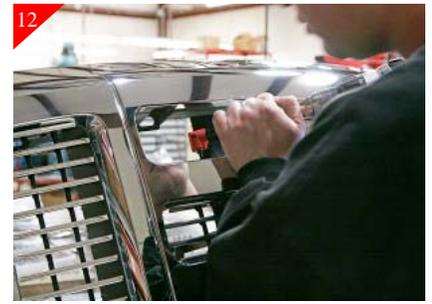
Repeat installation process for all openings with the exception of the **TOP BILLET GRILLE**. Mark and drill as in previous steps without attaching the billet grille. You will attach the billet grille after the stock grille shell has been placed back on the vehicle. The reasoning behind this is that you would not be able to reach the (7) plastic phillips head clips that you removed in step 2.
