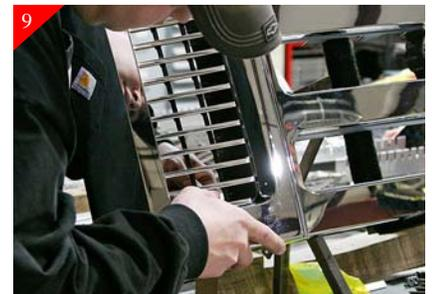
Attach billet grille using the supplied 10-32 x 1/2" and 10-32 nyloc nuts. Place bolts into mounting holes and secure with nyloc nuts.
