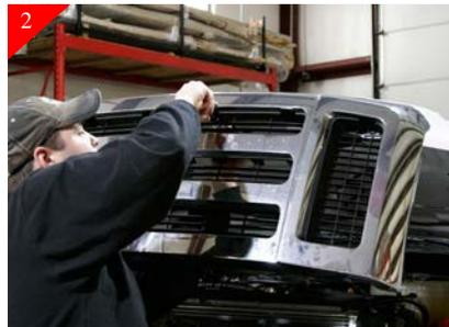
Locate and remove the (7) Plastic Phillips head screw clips that hold stock grille shell in place. They are located along top of stock grille shell. To aid in removing squeeze the backside of the clip to keep the screw threads engaged.
