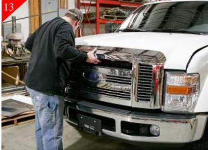
Place stock shell back on vehicle and snap the top back in place (Ref. step 3). Also replace the (2) 8mm bolts that were removed in (step 1).
