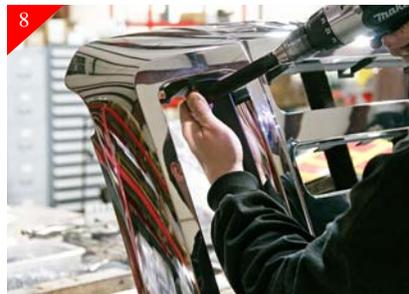
Drill just marked location using a 7/32" drill bit. Place billet grille back in opening and center.
