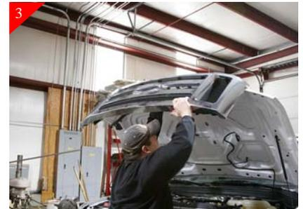
The stock grille shell is being held in place by snap clips across the top of the shell that clip into hood. Release these clips by supporting with one hand and with the other using a bumping motion or push towards the vehicle to release.
