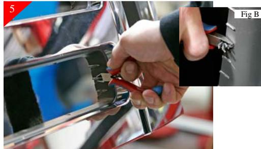
After all plastic centers have been removed clean up cut areas by using a pair of flush cut cutters and trim flush with stock shell as shown above. Flush cut cutters will allow you to cut as close as possible to stock shell without the need of sanding. Close up of trimming (Fig B).
