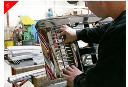
Starting with the wing portion place billet grille into opening and center. Make sure to push billet grille into opening and seat against the grey plastic in opening. Using a 90° scribe mark the hole locations for (1) of the mounting holes and remove the billet grille.
