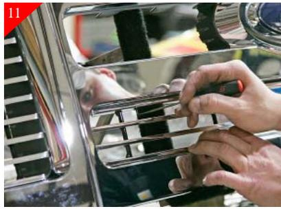
Locate the bottom billet grille by comparing the lengths of the (2) longest billet grilles. The bottom is the shorter of the (2). Place billet grille into opening and center. Using the same process as install of the wing billet grilles. Mark one end and remove billet grille. Drill just marked location using a 7/32" drill bit. Again using bolt to hold in place while marking the other mounting hole locations.
