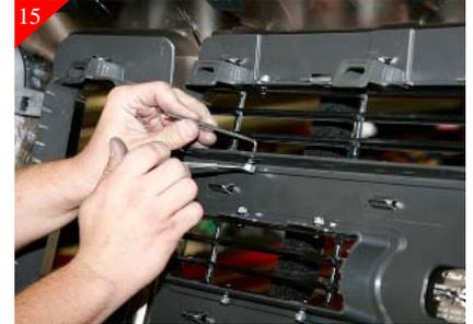
Place Top billet grille in place and center and attach using the supplied 10-32 x 1/2" and 10-32 nyloc nuts as shown above.
