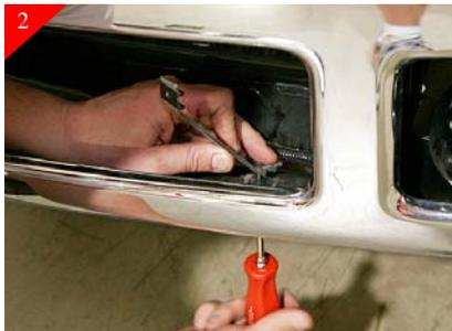
Next locate holes in stock bumper along the backside of bumper you will be utilizing these holes to attach the brackets from step 1. Using the supplied #8 x 5/8" Phillips head screws attach by screwing into the already placed u-clips as shown above.
