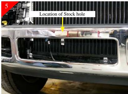
Next there is a hole located in the middle of bumper along the top opening. Attach bracket to this location by placing the supplied u-clip on hole then using the supplied #8 x 5/8" phillips head screw to fasten.
