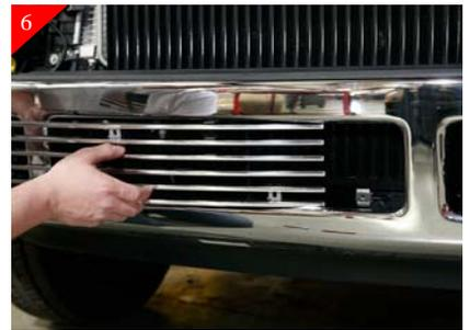
Place billet grille into opening, note that the billet grille goes behind the bumper opening. Start with placing one end into bumper opening and sliding it in behind the opening keep sliding until you are able to get the other end in place. Attach billet grille using the supplied #8 x 5/8" Phillips head screws.
