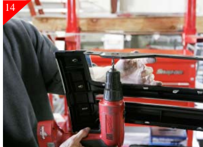
14 Using a 17/64" drill bit drill in the just marked locations.
