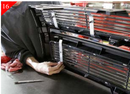
16 Place bottom portion of billet grille into opening and center. Attach bottom billet grille using the supplied 1/4-20 x 5/8" Bolts & 1/4-20 Nyloc nuts. Place bolt thru the mounting tab in billet grille and thru bracket and secure with the Nyloc nut as shown above.
