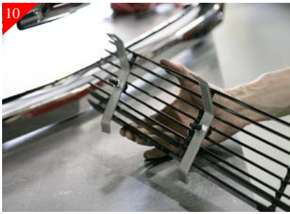
10 Attach the (4) brackets to top portion of billet grille using the supplied Bracket and 1/4-20 x 5/8" bolts & 1/4-20 Nyloc Nuts, as shown above.
