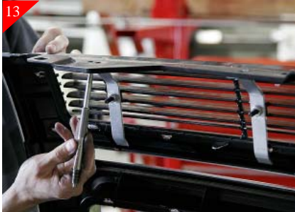
13 After aligning the billet grille using a scribe mark the (4) hole locations in brackets where it meets the shell as shown above. After marking remove billet grille from opening.
