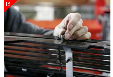
15 Place billet grille back in opening and attach using the supplied 1/4-20 x 5/8" Bolts, washers & 1/4-20 Nyloc nuts.
