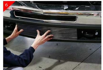
Place the supplied 10-24 x 2" bolts in the mounting tabs in billet grille. Now place the supplied spacers on the backside of the billet grille, slide the spacers on 10-24 x 2" bolts. Place billet grille back in opening and align with drilled holes. Push the 10-24 bolts thru the already drilled holes. Reaching from under front end place supplied washers on bolts and tighten using 10-24 Nyloc nuts.
