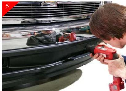
Drill just marked locations using a 1/4" drill bit.
