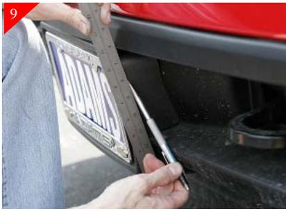
Start by using a straight edge as shown above. Using a scribe mark as shown, using the straight edge as a guide repeat for remaining side.
