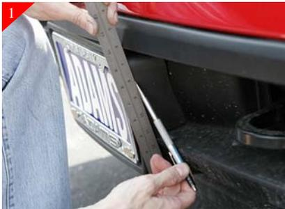
Start by using a straight edge as shown above. Using a scribe mark as shown, using the straight edge as a guide repeat for remaining side. You will be using this cut line later in the install to all re-attachment of the license frame. If your state doesn't require a front license frame you can skip cutting the license frame.
