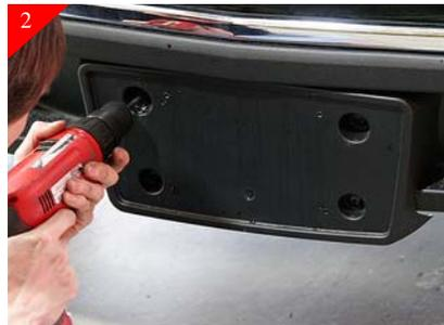
Start by removing the stock license frame. Do so by drilling out the rivets holding license frame in place using a 1/4" drill bit.
