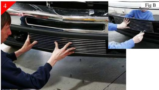
Place billet grille into opening and center. Align billet grille using the bottom of the bumper opening and the bottom bar in billet grille. Using a scribe mark the (4) mounting holes on the vehicle as shown (Fig B). Remove billet grille.
