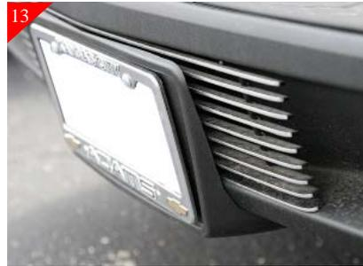
Attach license frame holder using the supplied 1/4-20 x 3/4" and washer on the head side of bolts and washer and 1/4-20 Nyloc nuts on backside as shown.
