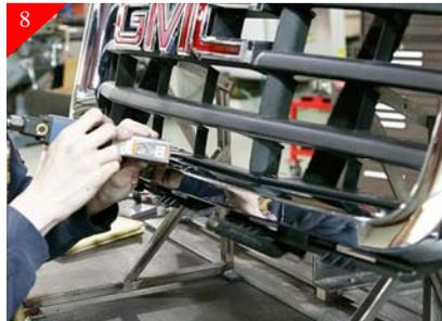
Again cut all horizontal and vertical attachment points flush with shell same as in previous step.
