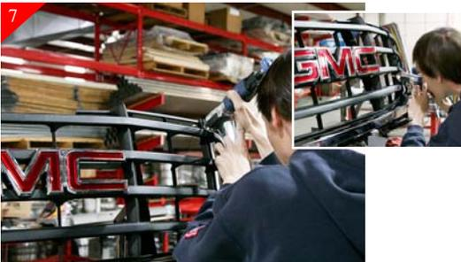
Move stock grille shell to a protected work surface. Using masking tape, tape the chrome portions of stock grille shell to protect during install. Using an air saw or other cutting device. You will be removing the center portion of the stock shell. Cut all horizontal and vertical attachment points flush with shell. Making sure to leave enough material to do finish sanding. **See (step 7-10) for more cutting images.**
