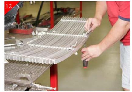
12 loosely attach the (2) bottom brackets using the supplied 1/4-20 x 1" Bolt and 1/4-20 Nyloc nuts shown above.
