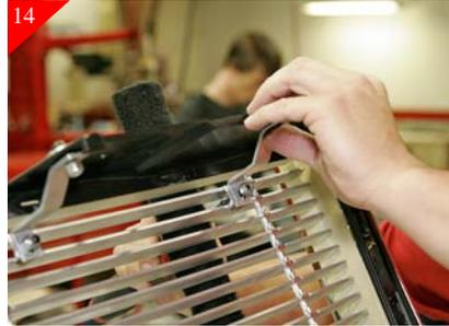
14 Now loosely attach the remaining (2) upper brackets to billet grille using the supplied 1/4-20 x 1" bolts & 1/4" Flat washers and 1/4-20 Nyloc nuts. The washer go on the head side of the bolt or on top of plastic.
