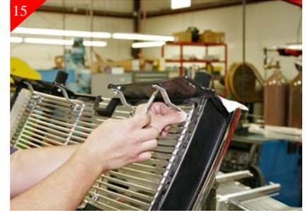
15 Using a scribe mark the mounting location where is meets the top of the shell as shown above.
