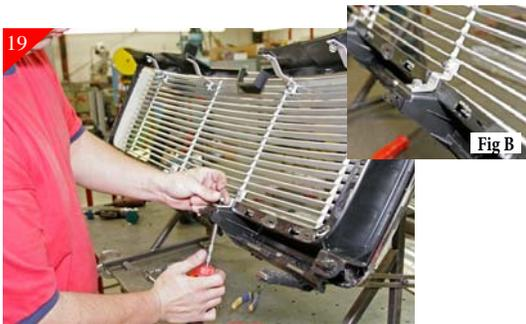
19 After drilling attach brackets using the supplied 1/4-20 x 1" bolts and 1/4-20 Nyloc nuts. Make sure the bottom brackets are butted against the black plastic (Fig B).
