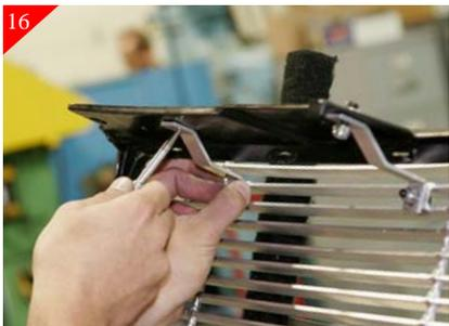
16 Repeat for other side--Using a scribe mark the mounting location where is meets the top of the shell as shown above.
