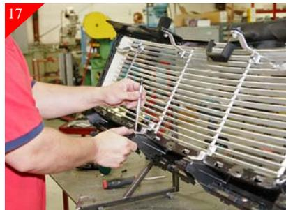
17 Using a scribe mark the mounting location where is meets the back of the shell as shown above. Make sure that the bottom brackets are firmly butted up against the black plastic shell before marking. Repeat for the remaining bottom bracket.
