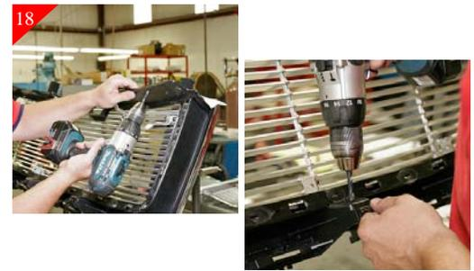
18 Drill all the just marked hole locations using a 17/64" drill bit.
