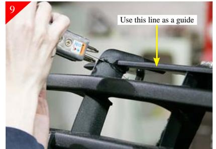
When you get to the top portion of the stock shell you'll notice the center will be open. Cut as shown above using the top portion of the stock shell or horizontal line as a guide.
