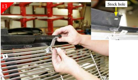
13 Loosely attach (2) upper brackets to the 2 inner mounting tabs in billet grille using the supplied 1/4-20 x 1" bolts and 1/4-20 Nyloc nuts. Now attach brackets to top of shell using the stock hole as shown above (Fig B), and also using the stock bolts. This will help hold billet grille in place while marking and drilling remaining mounting locations.
