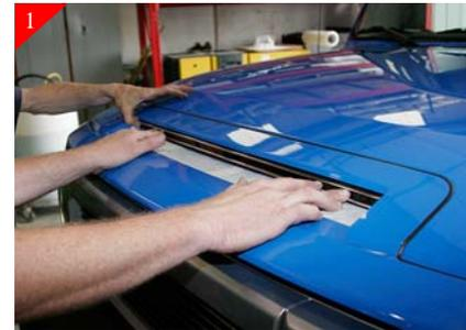
Tape hood using masking tape as shown above. This will help protect the hood during install. Next place billet CNC machined hood insert into opening and center.
