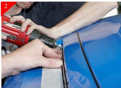
After centering check alignment of insert. Starting with 1/16" drill bit and then moving to a larger 3/8" drill bit as shown above drill ONLY the outer (2) mounting holes. After drilling attach using the supplied 10-32 well nuts and 10-32 x 5/8" bolts. Place well nuts into just drilled locations and seat against the hood opening then attach using the 10-32 x 5/8" bolts.
