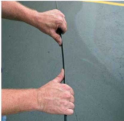
Your Insert needs to follow the contour of your hood. It maybe necessary to form the insert slightly by bending as shown above due to shipping. Be very careful around the mounting holes during this process as it may bend to much and or crack the mounting hole.
