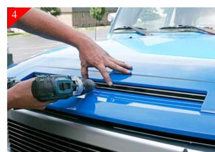
After drilling the center mounting hole. Attach CNC machined grille using the supplied 10-32 x 5/8" bolts and 10-32 well nuts. Install is complete
