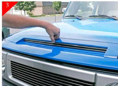
Next you will be preparing for drilling the center mounting hole. Do so by pushing slightly down on the center portion of the insert as shown. This will align the insert properly with hood opening. You will need to hold the insert in this position during the first drilling process. Using 1/16" drill bit drill the center mounting hole. Now remove the CNC machined grille from opening and finish drilling the center mounting hole using the larger 3/8" drill bit.
