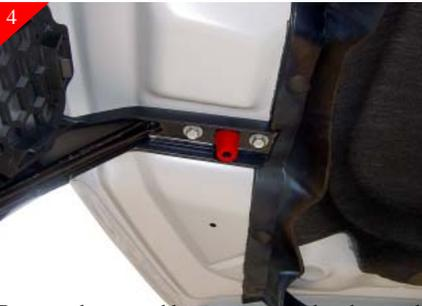
Remove the two rubber stops on the brackets and **SAVE** them. They will be reinstalled. Move to a protective work surface.
