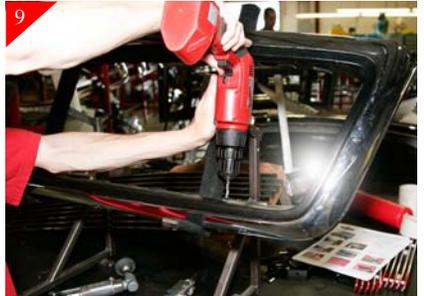
Drill all just marked locations using a 7/32" drill bit.
