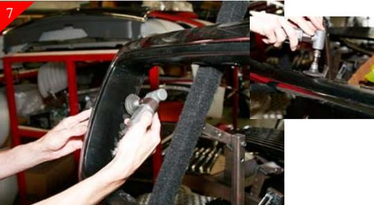
Using a grinder or sanding block sand the cut areas smooth for driver and passenger side of stock shell. Now sand the top and bottom of the stock shell just to clean up cut areas. Do not sand flush! These raised areas are needed to register billet grille into opening and will not be seen after billet grille is installed.
