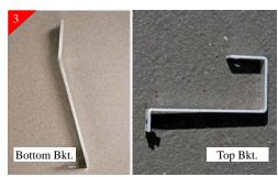
The above brackets are orientated the correct direction for install. Loosely attach brackets to billet grille using the supplied 10/32 x 5/8" bolts and nyloc nuts. Rotate the brackets around so that you can place the billet grille into opening. Rotate the brackets back in place and tighten.
