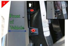
Next you will be attaching the top bracket to the factory 8mm bolts shown above. (Please Ref next step for diagram of attachment of brackets). Next locate the factory 8mm bolts on lower valence and remove, then attach the bottom bracket to these factory bolts. (Please Ref next step for diagram of attachment of brackets).
