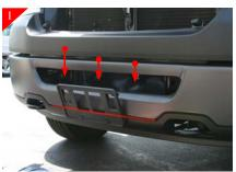
Remove the (5) 8mm bolts by reaching thru the front opening of vehicle. Area of bolts to be removed shown above in RED.
