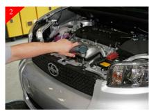
Remove stock shell by removing (2) plastic rivets on each end of the stock shell. Then remove (2) 10mm bolts along top of stock shell shown above.
