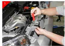
Locate supplied upper brackets and place u-clip on brackets as shown above. Attach upper brackets by placing brackets in the (2) outer most stock mounting tabs as shown then place a supplied U-clip on the under side and attach using the supplied #8 x 1" phillips head screws as shown above.
