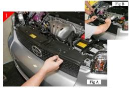
Remove plastic core support cover by removing the plastic rivets across top of core support as shown (Fig A). Use of a small regular screwdriver will aid in the removal of the rivets. (Fig B) remove support cover.
