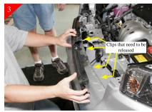
Reaching down behind stock shell release clips along bottom of stock shell. Stock shell will be free at this point.
