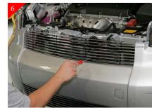
Place billet grille into opening and center. Using the supplied #8 x 5/8" phillips head screws attach billet grille to brackets.
