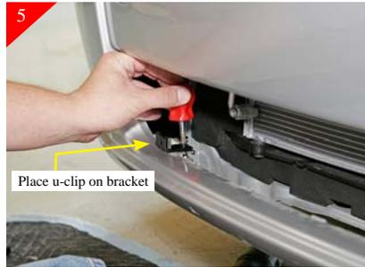
Place supplied u-clips on the supplied lower bumper brackets (Long) as shown. Attach bracket to vehicle using #8 x 5/8" phillips head screws as shown above. A short or stubby screwdriver will be needed to tighten. Repeat process for remaining bumper brackets. The (Short) bumper brackets attach to the upper portion of the bumper opening.
