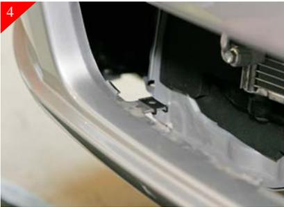
Place supplied u-clips on ends of the plastic bumper opening tabs as shown above. There are (4) total (2) on the bottom and (2) on the top.
