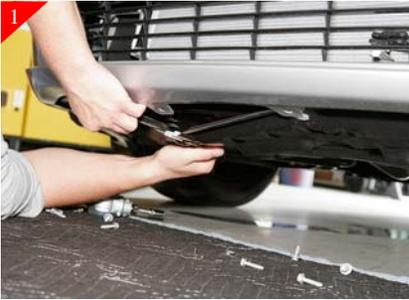
Remove splash guard from under front end of vehicle. Do so by removing the 10mm bolts holding splash guard in place. Take note of bolts for installing later. The front row of bolts are the longer screw type bolts and the back row are shorter.
