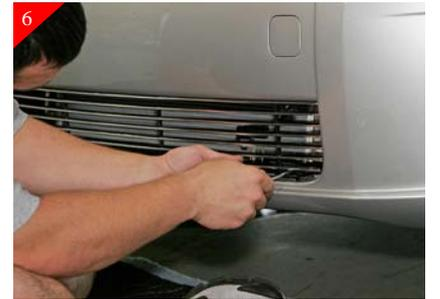
Place billet grille into opening and center. Attach billet grille to brackets using the supplied #8 x 5/8" phillips head screws. Install is complete. Re-install splash guard.
