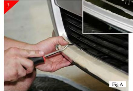
Remove stock bumper insert by using a regular screwdriver to release insert (Fig A). (Fig B) Shows after insert has been removed to show plastic clips that hold stock insert in place.
