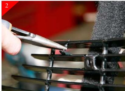
2 First you will be attaching sheet metal trim across top of billet grille. Starting on the right side of the billet grille, place supplied OEM style rivets up thru mounting holes as shown. Using a pair of needle nose pliers will aid in the placement of rivets.
