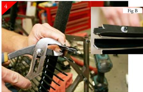
4 Fasten sheet metal trim by using a large pair of channel locks as shown. Try and catch the washer with channel locks so it holds in place with securing rivets. (Fig B) shows attached trim.
