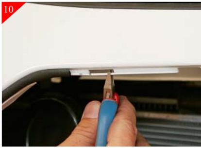
Using a pair of straight cut dykes or cutters, cut the inner most slot as shown above. This will allow for clearance for the already placed rivets. So the billet grille will be able to slide into place.
