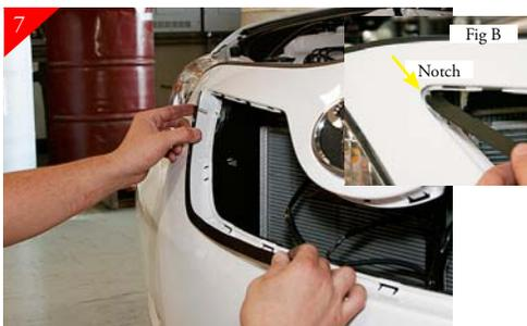
7 Locate the supplied surround trim pieces (left & right). Place surround trim as shown with notch going up in the top corner of stock grille shell as shown (Fig B). The mounting studs go thru holes where stock clips fastened.
