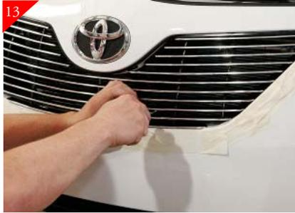
Place billet grille into opening and center. Attach billet grille by using the supplied #10-24 x 5/8" bolts and 10-24 nyloc nuts attach to the already placed upper and lower brackets. Do so by reaching down behind the stock grille shell and tighten.
