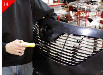
After Attaching billet grille you will need to attach the center bracket that helps align the logo area of stock shell with billet grille. Do so by attaching supplied bracket to mounting tab located in middle of the billet grille. Attach using 10-24 x 5/8" bolt and 10-24 Nyloc nut and tighten as shown. After attaching bracket remove adhesive cover and tape.
