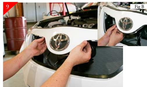
9 Next you will be attaching the supplied rubber molding. Start by test fitting the rubber by centering the rubber around logo area of opening. This to get an idea as to where the rubber needs to be. Then peel the adhesive backing off and starting on one end of the rubber attach and slowly work your way around emblem area without pulling or stretching the rubber molding (Fig B) let it naturally follow contour of the logo area.
