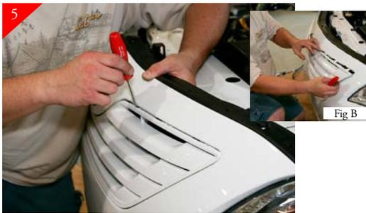
5 Next you will be removing the center portion of stock shell. Do so by releasing the clips that surround grille shell. Using a regular screwdriver and pushing slightly from the backside will aid in the release of the clips. Take time in releasing clips so as not to scratch painted surface. Continue working around the outside of stock grille shell releasing clips until center is free (Fig B). There are 22 clips total.
