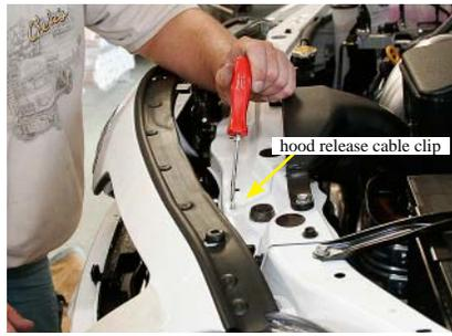
Release the hood release cable by using a regular screwdriver and push clip out of hole. This is just to move the cable out of the way for installing the upper brackets.
