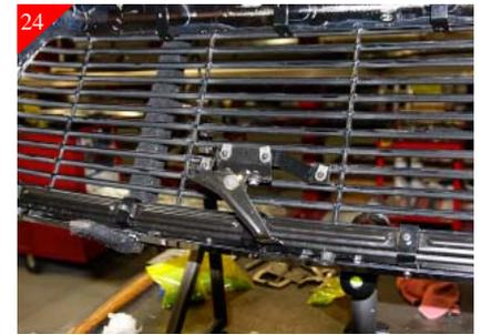
24 Attach stock hood release lever to this bracket using the supplied U-clips and 10-24 x 5/8" soc head bolts as shown above.
