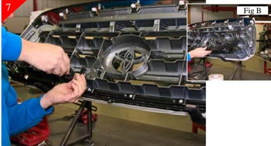
Locate the Phillips head screws holding the steel brace along bottom of stock shell shown above and remove.
