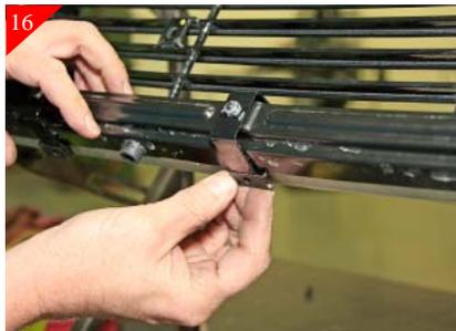
After drilling all hole locations place supplied U-clips on the brackets as shown.
