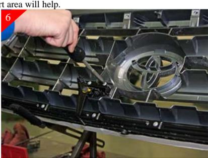
Remove the Phillips head screws holding hood release lever in place. Keep lever to be re-installed to billet grille later in the install.
