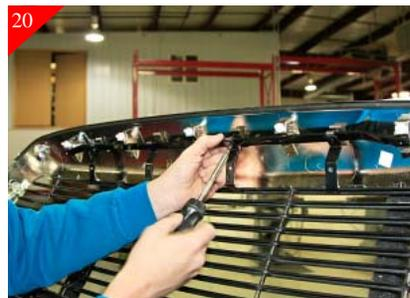
Locate and place the supplied top cross bar as shown. Then attach brackets to the top bar using the supplied U-clips and 10-24 x 5/8" philips head screws.
