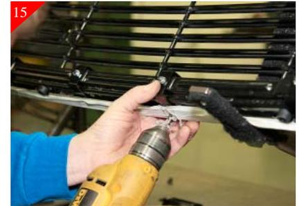
Drill all the just marked hole locations using a 3/16" drill bit.
