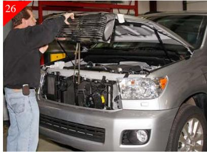
26 Place the grille shell back on the vehicle. Align the snap clip across the top of the shell with the hood and snap in place. A slight bump with the palm of your hand where the clips are will seat in place.
