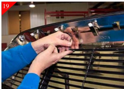
Attach brackets to billet grille using the supplied 10-24 x 1/2" soc head bolts and 10-24 low profile nyloc nuts. See previous step for orientation of brackets.
