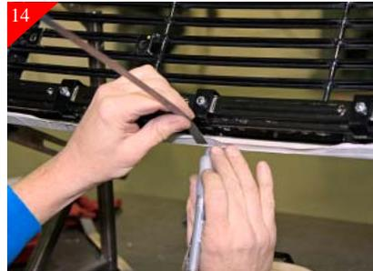
Next you will laying out the holes to be drilled in the stock shell. Do so by using a straight edge to trace the edges of the bracket onto the tape on the stock grille shell as shown above. Then measure 1/2" from the backside of the grille and mark a center line to be drilled.
