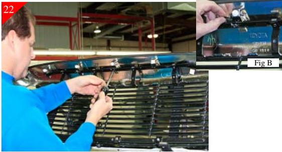
22 After drilling all hole locations, place supplied U-clips as shown in (Fig B). Attach using the supplied 10-24 x 5/8" Phillips head screws.
