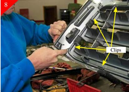
Starting on one end of the grille shell you will be releasing the clips that hold the center section in place. Using a small regular screwdriver to help in releasing clips will be necessary. Once you get several clips released the rest will be much easier.
