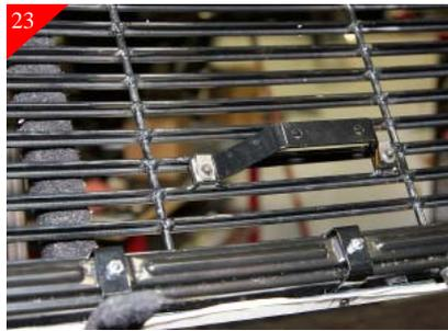
23 Locate and attach hood bracket to the billet grille using the supplied U-clips and 10-24 x 5/8" soc head bolts. Place the supplied U-clips on the hood release bracket and attach with bolts. Attach stock hood release lever to this bracket.
