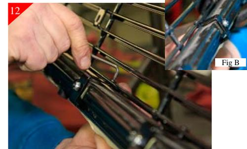
With the bracket under the bar of the billet grille attach using the supplied 10-24 x 1/2 soc head bolt and 10-24 low profile nyloc nut. When tightening use of a ball end Allen wrench or a shortie as shown above will be necessary.
