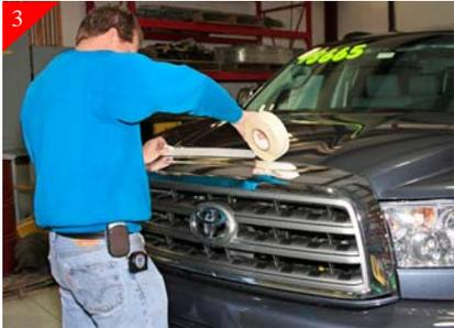
Using masking tape, tape off the hood area just behind the chrome of the stock grille shell. This will protect the hood when removing the grille shell. Also to help hold the hood in a better position for removing grille shell use of a bungee cord or a piece of rope hooked to the hood latch and core support area will help.
