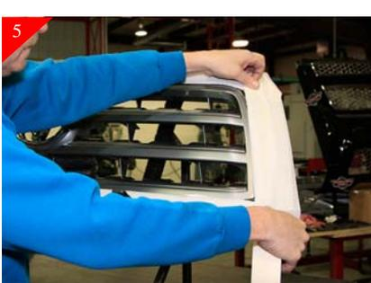
Move stock grille shell to protective surface. Using masking tape, tape the face of the grille shell to protect during install of billet grille. Flip stock shell over face down.
