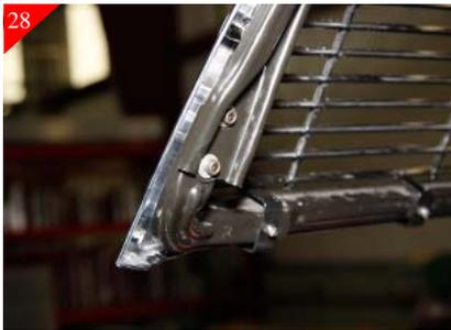
28 Next you will be attaching the bottom steel brace to the vertical steel brace coming off the hood. Attach using the supplied 1/4-20 x 3/4" soc head bolt and 1/4" washer followed by washer and 1/4-20 Nyloc nuts. Washers go on both the head side and backside. Use of an open end wrench will be necessary in securing. Install is complete.
