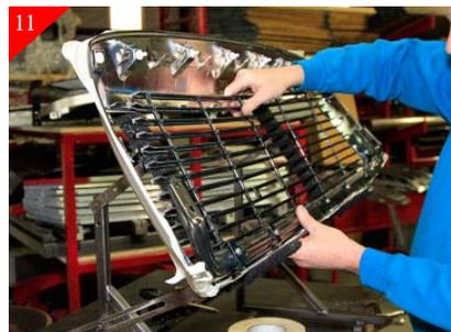
Place billet grille into opening and center. Move steel brace to shell and lay in place and center. Next you will be attaching the steel brace to the 2nd bar from the bottom in billet grille using the brackets along steel brace.
