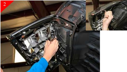
Next locate the (10) 10mm bolts on the backside of the stock grille shell and remove. With these removed the only thing holding the grille shell in place is snap clips along the top of the hood area.
