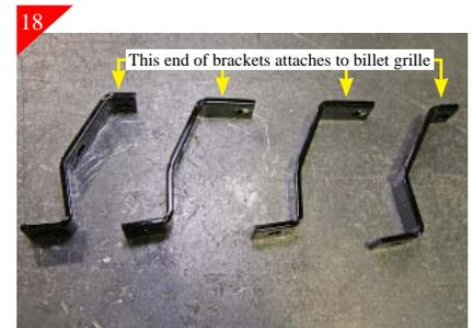
Located the supplied upper brackets. Brackets shown above are laid out in the correct attach order. With the (2) outside brackets attaching to the outside and the (2) middle one going to the middle. The hole in the end of the bracket closest to the edge will attach to the billet grille.
