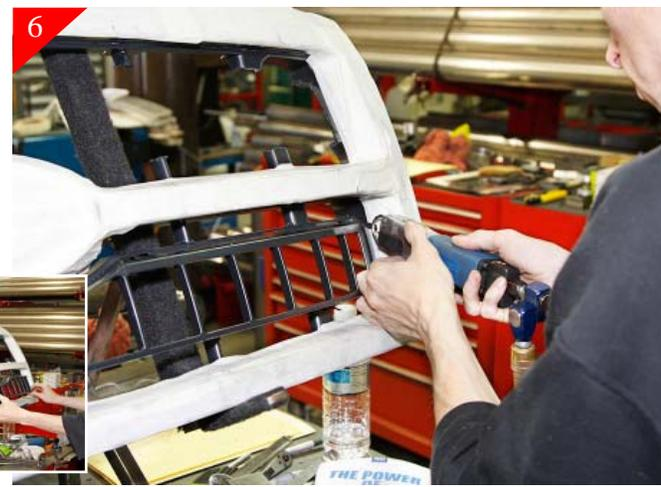
Again using the same method as in step 2. Using a cut-off wheel or air saw cut the vertical attachment points, leaving plenty of material to come back and clean up cuts and to do finish cutting and sanding.
