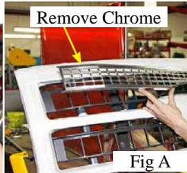
Now you will be separating the chrome Facia from the stock grille shell (Fig A). Do so by releasing the clips on the backside of the stock grille shell. Use a regular screwdriver to lift the plastic clip up to release as shown (Fig B).
