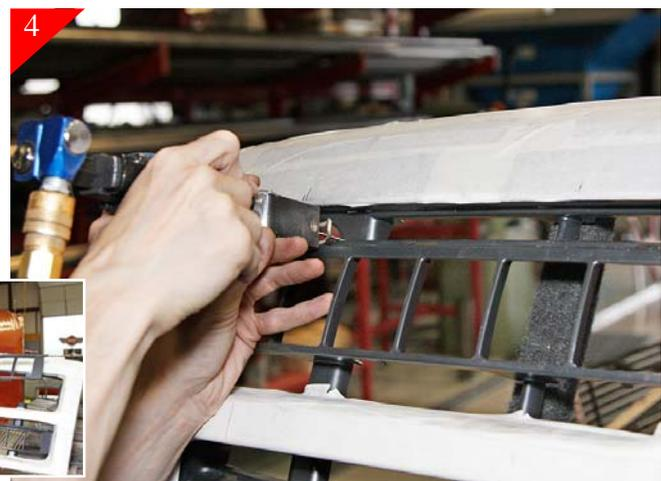
With the chrome facia removed you can now remove the remaining plastic center. Using a cut-off wheel or air saw cut the vertical attachment points, leaving plenty of material to come back and clean up cuts and to do finish cutting and sanding.
