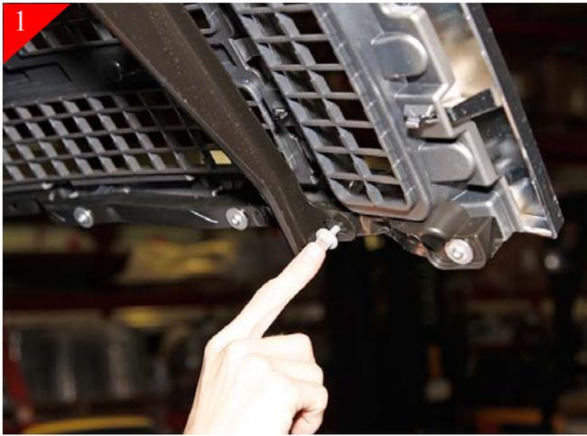
Open hood and remove the (2) 10mm bolts along the bottom outside of the stock grille shell holding the stock grille shell in place.
