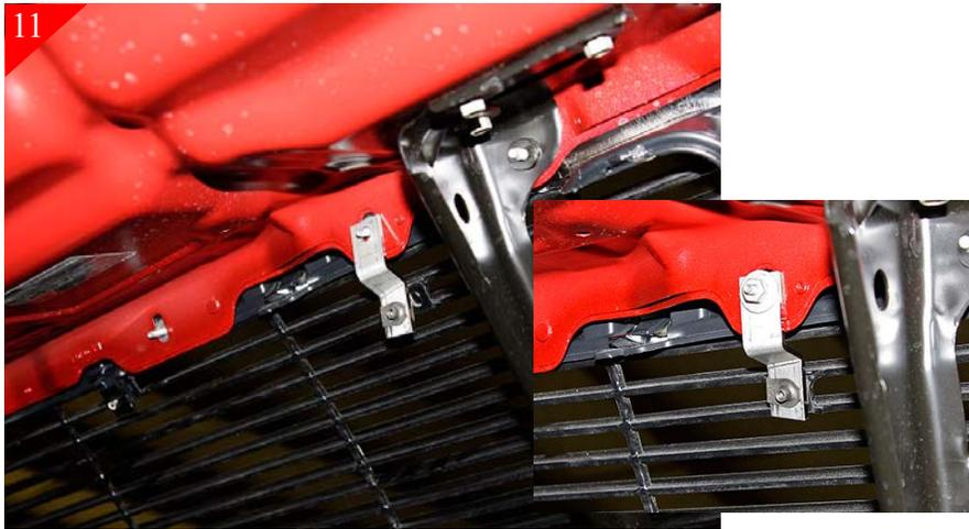
Now locate the remaining brackets and place the supplied 10-24 u-clips on the end of the bracket with a angle bend as shown above. Next place grille shell back on vehicle. Now place the bracket as shown on the mounting stud of the grille shell. Using the supplied 10-24 x  $\frac{5}{8}$ " bolts attach bracket to billet grille. Repeat more remaining side of the billet grille.
