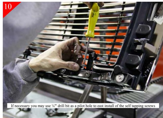
Next locate the (2) "L" Brackets and place the supplied 10-24 u-clips on the long end of the brackets shown above. Attach brackets to the 2 lower outer mounting tabs in billet grille using the supplied 10-24 x  $\frac{3}{8}$ " bolts and attach to the just placed u-clips. Next using the supplied self tapping screws attach the short end of the brackets to the steel framing as shown.
