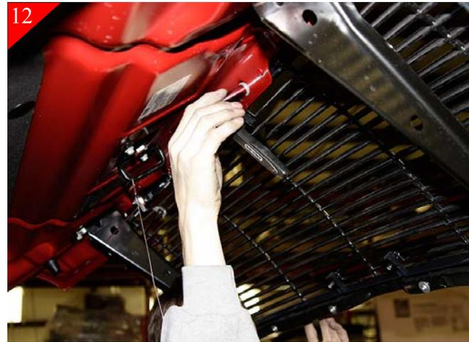
Continue with the re-attachment of the grille shell using the stock hardware removed in steps 1 and 2. Check all hardware and fasteners. Install is complete.
