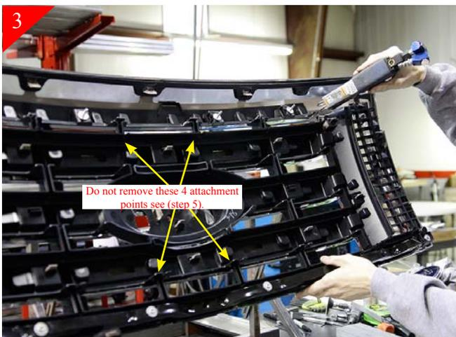
Next you will be removing the center portion of the stock grille shell. Using an air saw cut the vertical attachment points of the grille shell shown above. **DO NOT START WITH THE MIDDLE 2 ATTACHMENT POINTS THESE WILL BE ADDRESS IN STEP 5 OF THE INSTALL.**
