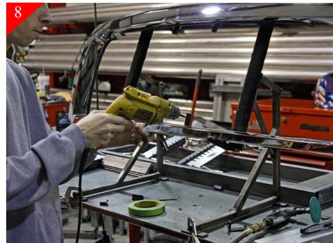
After marking mounting locations remove billet grille from opening. Drill the just marked locations starting with a pilot hole using a  $\frac{1}{8}$ " drill bit. Next using a  $\frac{1}{4}$ " Drill bit re-drill locations.
