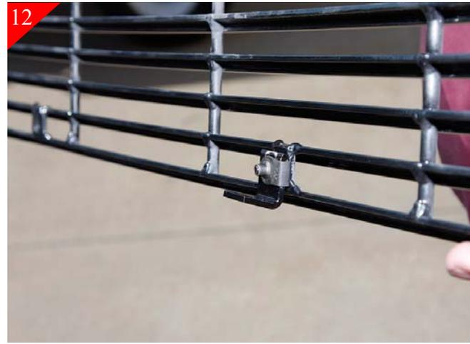
Locate the supplied bottom brackets and place supplied 10-24 u-clips on the long end of bracket and attach bracket to billet grille using 10-24 x 5/8" as shown above there are (3) brackets along the bottom.
