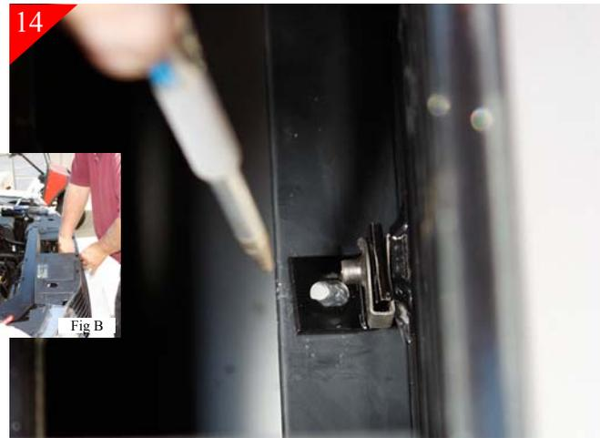
Now reaching down on the backside of the billet grille using a scribe mark the (3) bracket locations of the just placed bottom brackets (Ref step 12). After marking hole locations remove billet grille from opening. Also remove the brackets from the billet grille.
