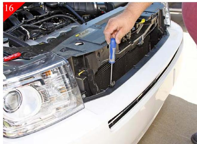
Next attach the bottom bracket that you removed (Ref step 14) to the just placed u-clips. Attach using the supplied 10-24 x 5/8" bolts as shown above
