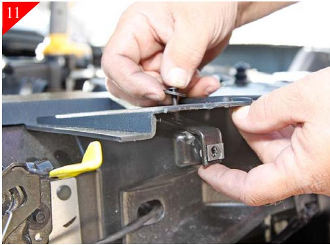
Next locate the supplied upper brackets and place supplied u-clip on the bent end of bracket. Then place on top of the just placed well nut in between the plastic core support cover as shown. Attach bracket using the supplied washer and 10-32 x 1" button head bolts. Snug bolts in place do not fully tighten at this point.
