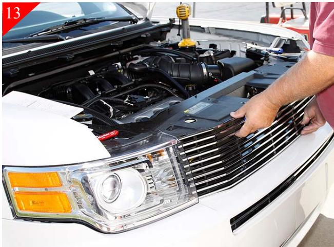
Place billet grille into opening and center. Push billet grille against the small vertical plastic along the bottom of opening (Ref step 8). The plastic core support cover seats in the top channel of the top bar in billet grille. Check alignment around billet grille.
