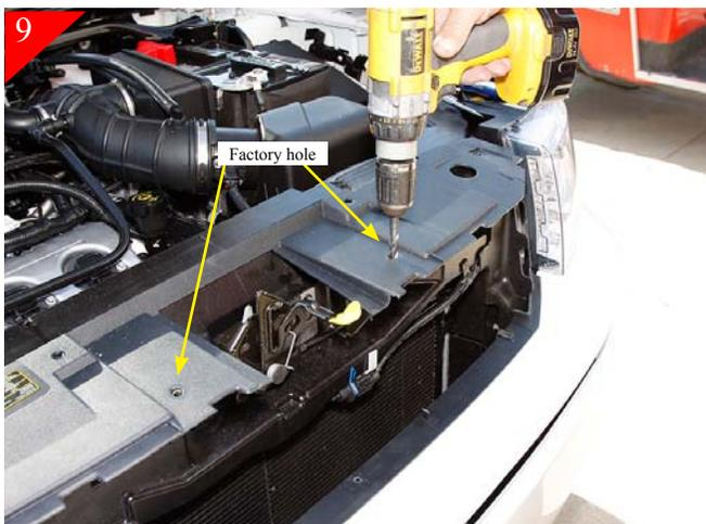
Next locate the (2) factory holes located on each side of the hood release. Using a  $\frac{3}{8}$ " drill bit drill down through plastic into the steel support below.
