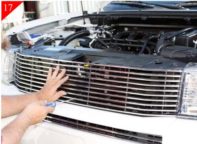
Place billet grille back into opening and attach using the supplied 10-24 x 5/8" bolts. Make adjustments as necessary and tighten all hardware.
