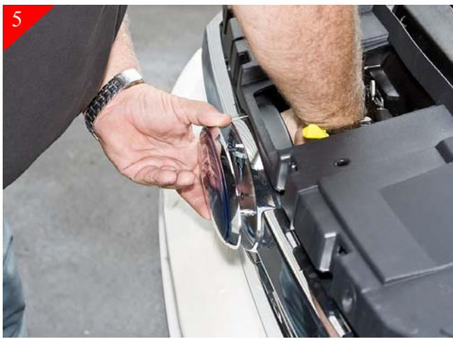
You will also need to remove the Ford emblem by removing (2) 10mm nuts from back side of shell. Chrome portion of the stock grille shell will be free at this point.
