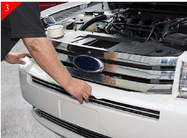
Tape the front end of the vehicle and the headlights using masking tape to protect the vehicle during install as shown above.
