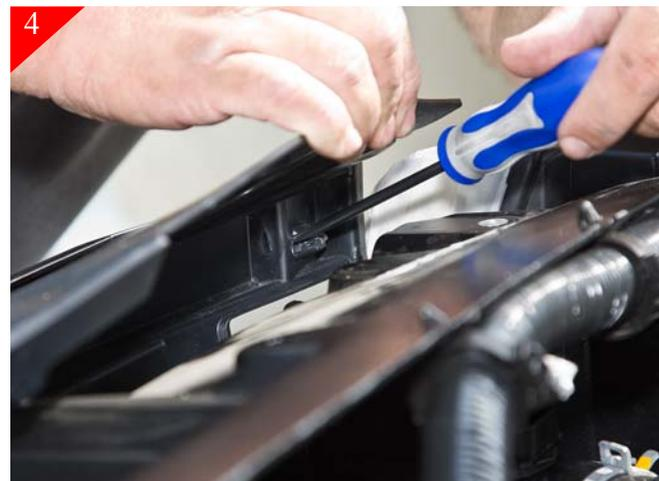
Next you will be removing the chrome portion of the stock grille shell. Do so by reaching behind the stock shell and releasing the clips holding chrome front using a large regular screwdriver to release. There are (6) clips located along the top of the shell, and (4) clips located across the middle of shell, and (6) along the bottom of the shell.
