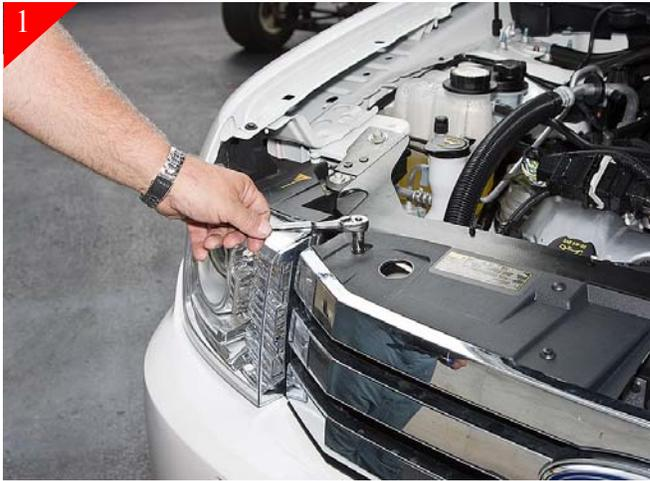
Remove (2) 10mm bolts opposite from each other located on top of the plastic core support cover shown above.
