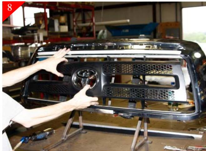
With all Attachment points cut the stock center will be free at this point, and remove.
