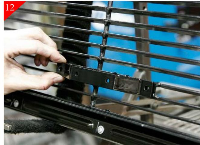
After attaching billet grille you will need to attach the hood release brackets to billet grille. Attach supplied bracket shown above to the mounting tabs in billet grille using the supplied 10-24 x 5/8" bolts and 10-24 Nyloc nuts.
