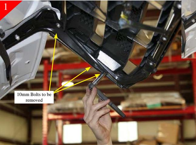
First start by opening the hood on your vehicle. Next there are the (3) 10mm bolts on both the driver and passenger side of the truck that attach the steel brace and the stock grille shell together that need to be removed (Fig A & B).
