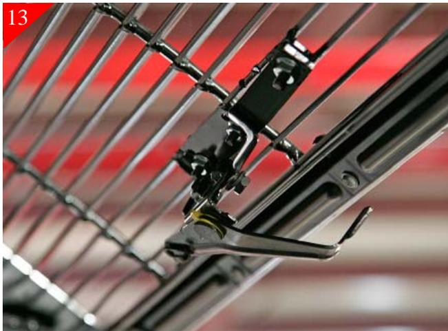
Now using the stock bracket that was removed in step 4, attach to the just placed bracket in step 12 using the supplied 10-24 x 5/8" and 10-24 Nyloc nuts.
