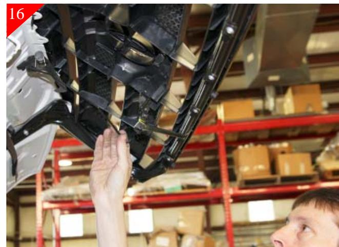
Re-attach hood rod that was detached in step 3. Check alignment of stock grille shell before closing hood. Install is complete.
