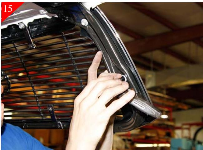
Attach the outer portion of the grille shell to steel braces using the stock 6mm bolts.
