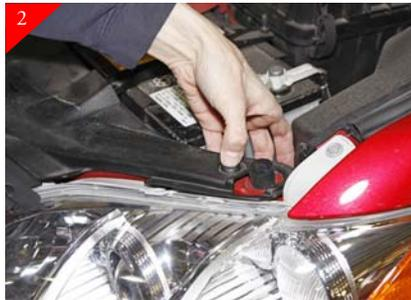
Remove the plastic core support cover by removing the (6) plastic rivets shown above. Remove the rivets by pushing on the center portion of the rivet and remove plastic. This allows you to reach behind the stock grille shell.
