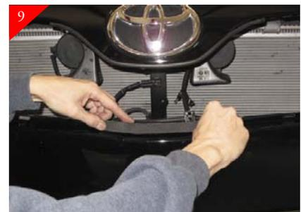
Locate the short piece of the flat molding. Test fit molding in between the two lower brackets trim in necessary. Remove adhesive backing and place as shown above.
