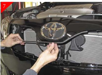
Next you will be attaching the supplied round rubber molding. Start by test fitting the rubber by centering the rubber around logo area of opening. This to get an idea as to where the rubber needs to be. Then peel the adhesive backing off and starting on one end of the rubber attach and slowly work your way around emblem area without pulling or stretching the rubber molding let it naturally follow contour of the logo area.
