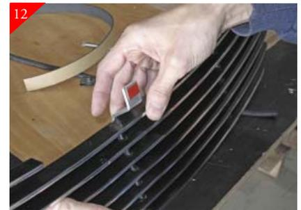
Attach the center bracket that helps align the logo area of stock shell with billet grille. Do so by attaching supplied bracket to mounting tab located in middle of the billet grille. Attach using 10-24 x 5/8" bolt and 10-24 fender clip and tighten as shown. After attaching bracket remove adhesive cover and tape.
