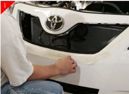
Tape front end of vehicle using masking tape to protect during install.
