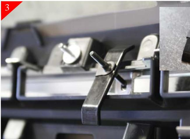
Next you will be attaching the (2) center brackets. Place supplied u-clips on brackets as shown above. Push the supplied 10-24 x 2" bolts through the 2 upper center mounting tabs in billet grille. Next place the brackets and rotate as necessary to catch the backside plastic and then tighten. With all brackets in place check alignment and then tighten all hardware.
