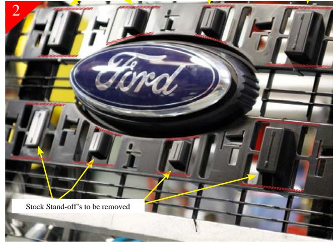
Next you will be removing all of the stand-off's that are behind the stock chrome strips that were just removed. Using the red lines above as guides you will be cutting from pocket to pocket which are on the left and right side of the stand-off's.
