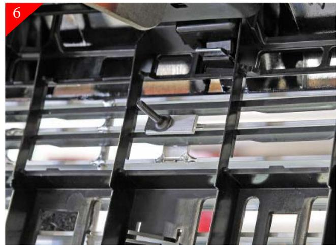
Place the billet grille into the opening and center. Now using a screwdriver rotate the tabs horizontal so that they will pass thru the stock grille opening repeat for all tabs.
