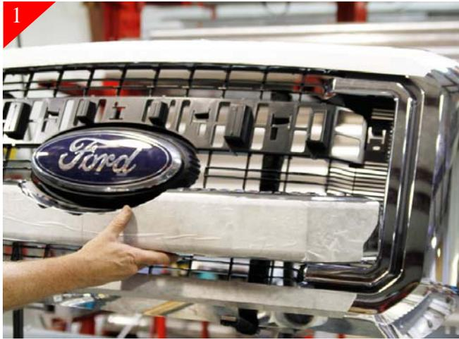
First you will be removing the (2) large horizontal stock chrome overlays from your vehicle. Do so by releasing the clips from the backside.
