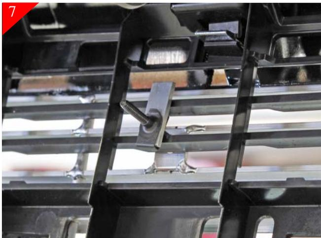
Utilizing 2 screwdrivers will be necessary. Using one on the bolt head and the other to rotate the brackets so that the u-clip is toward the bottom and then tighten in place.
