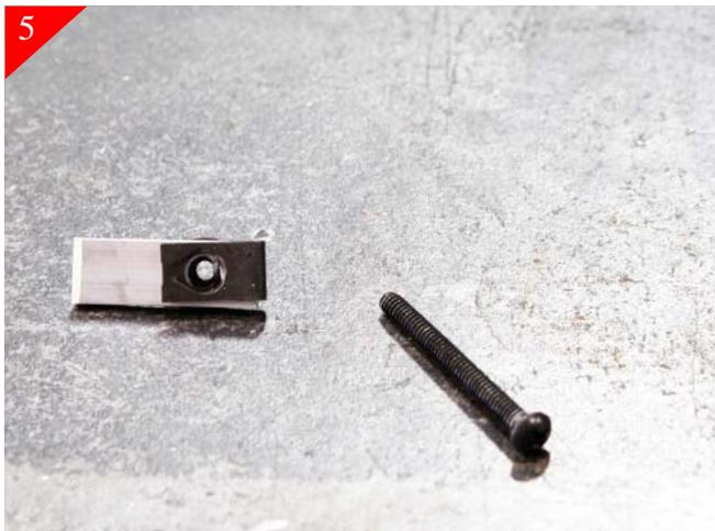
With all stand-off's removed now its time to install the billet grille. Locate the (8) supplied rectangle tabs and the (8) 10-24 u-clips and place the u-clip on the hole end of the tab as shown above repeat for all tabs. Now place the 10-24 x 2" bolts thru the mounting tabs in billet grille and just start to thread the tabs onto the bolts repeat for all mounting locations.
