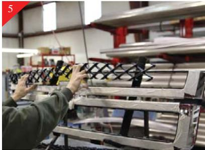
After cutting all attachment points remove top section from stock shell as shown.
