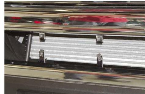
3. Next attach brackets into bumper opening using the stock bolts and stock locations to secure brackets in place. The bend in the brackets go to the inside toward Trans and Intercooler. See (Fig C).
