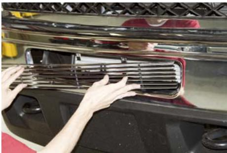
4. Place billet grille into opening placing one in first and pushing past the opening and then bring the opposite end in and slide back. Align mounting tabs in billet grille with the brackets and secure with the supplied 10-24 x 1" bolts. Tighten bolts without over tightening. Note: A drop of red/blue loctite on the bolt threads will significantly reduce the chance of bolts backing out due to road vibrations.
