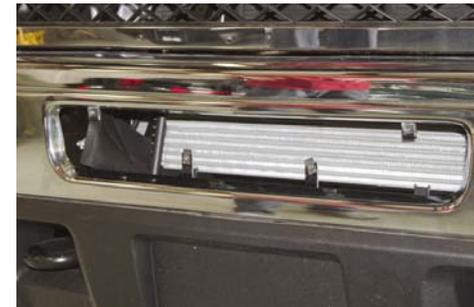
3. Next attach brackets into bumper opening using supplied bolts and stock locations to secure brackets in place. Place washer on the top side of the upper brackets. Next using the supplied u-clips use as a nut on top. The bend in the brackets go to the inside toward Trans and Intercooler. See (Fig C).
