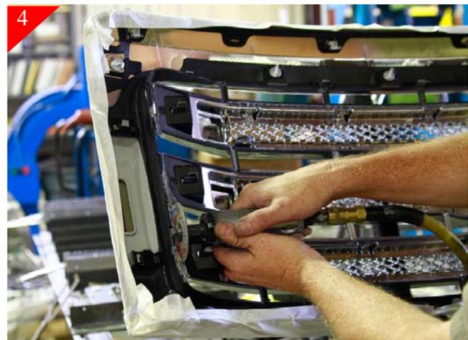
Next you will be making the last verticle cuts that will remove the center portion of stock grille shell.
