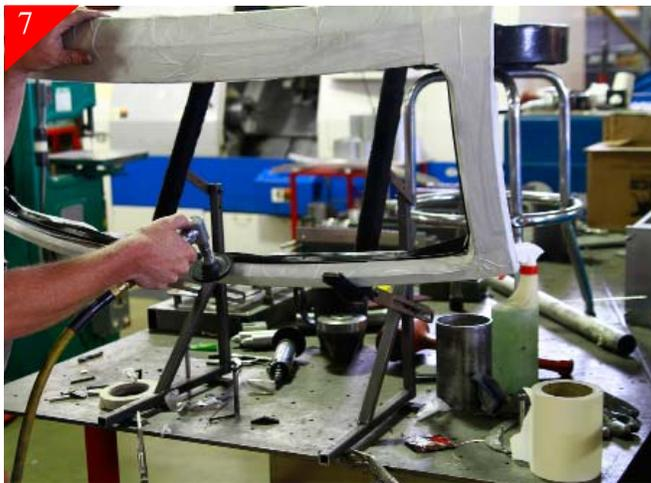
Using a sanding block or grinder cleaning up all the cut areas.
