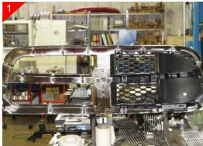
Start by removing stock grille shell from vehicle. Then move grille shell to protective work surface. With grille shell face down remove the plastic from the backside of the chrome shell. Do so by using a regular screwdriver to release the clips holding plastic to stock grille shell. Repeat for remaining side.
