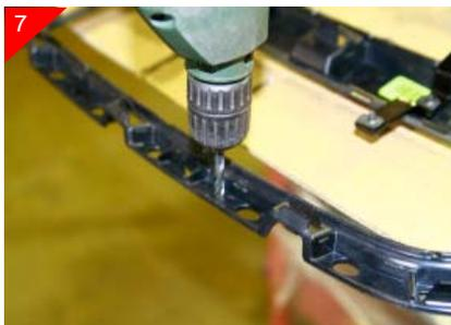
With all hole locations marked remove billet grille from stock grille shell and also unsnap and remove the black plastic for drill purposes. Using 1/4" drill bit, drill all just marked locations.
