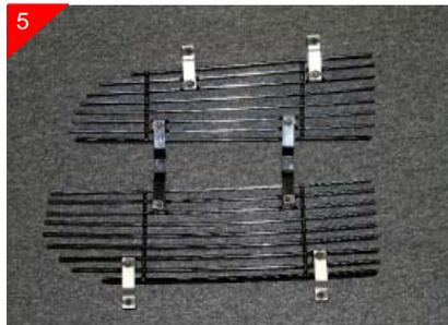
With all cross hatch sections removed and sanded smooth. Next you will be marking hole locations to drill for the installation of brackets. Start by laying billet grilles face down then attaching brackets to billet grille as shown above. This attaches the top and bottom grilles together.
