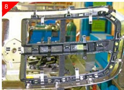
Next remove brackets attached to billet grille and place one at a time in the correct location using a 10-24 u-clip to attach brackets as shown. With all brackets attached to the black plastic snap back in place making sure that grille snaps in at all locations. Repeat all steps for the remaining side of grille
