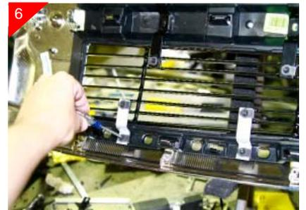
With stock grille shell face down place billet grilles in from the backside and center into openings. Using a scribe or sharpie mark the bracket locations where it meets the black plastic shown above. Mark all hole locations for the top and bottom billet grille.
