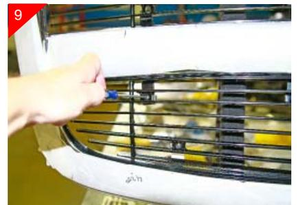
Turn stock grille shell face up and place billet grille into opening and attach using the 10-24 bolts. A small drop of blue loctite will insure nothing comes loose due to road vibrations. With all billet grille attached reattach stock shell to vehicle.
