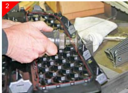
Next you will be removing the cross hatch section from the plastic just removed from shell. Using a cut-off wheel or air saw cut where the cross hatch meets the outer part of the shell leaving some material to come back and sand smooth. Repeat for remaining other cross hatch areas.
