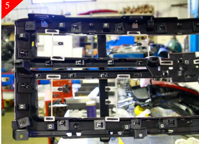
Referring to step 4 place brackets as shown. Repeat for remaining side of grille.
