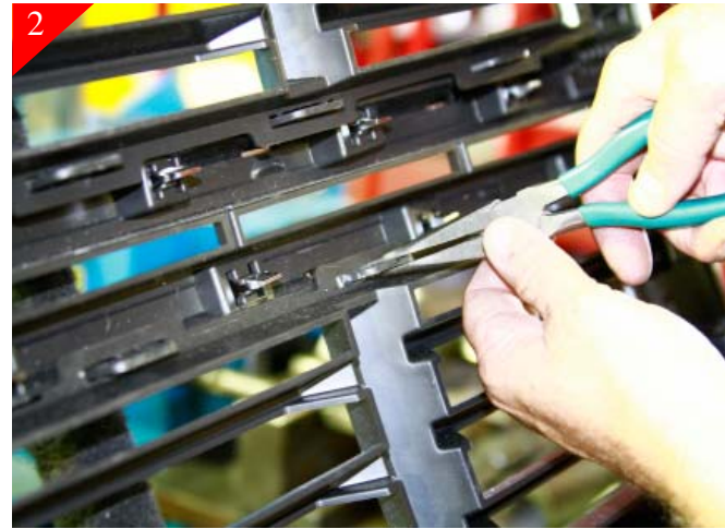
Next remove the black stock inserts from shell by pushing down on the clip to release. Remove both top and bottom portion.
