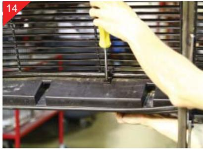
Next using a 1/4" drill bit, drill the just marked locations. Place billet grille back into opening and center. Attach both the top and bottom of the billet grille by placing 10-24 uclip on the underside for the bottom or topside for the top. Bottom is shown above.
