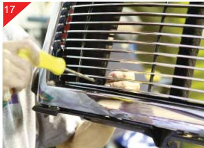
Attach brackets to stock shell using 10-24 uclips and 10-24 x 5/8" bolts placing the uclip on the underside for the bottom and topside for the top. With brackets attached place billet grille into opening and attach billet grille to the just placed brackets.
