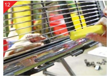
With grille placed into opening attach bottom center bracket to billet grill using 10-24 uclip and 10-24 x 5/8" bolt. Next you will be marking the hole locations for the attachment point of the brackets. You will mark and drill the top and bottom holes and then attach billet grille. This will help with marking and drilling of the remaining locations.
