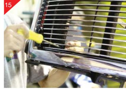
With the center points of the billet grille attached, next you will need to attach the remaining top and bottom brackets to the billet grille and then following previous steps for marking and drilling hole locations.
