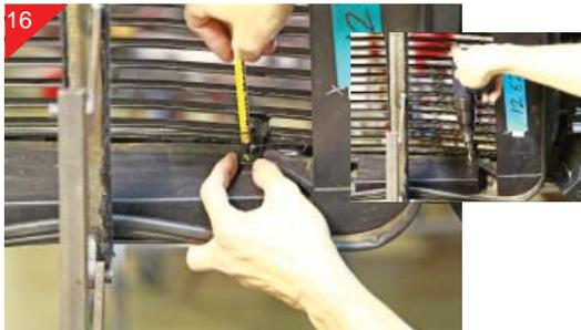
With all brackets attached using a sharpie mark all remaining hole locations. After marking all holes remove billet grille and drill just marked locations.
