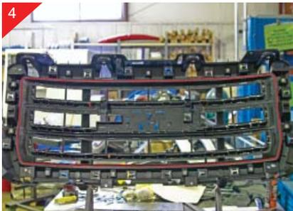
Move chrome portion of the shell aside. Next you will cutting or removing the center portion of the shell (black plastic). Using the red line as a guide cut along using a cut-off wheel or air saw leaving about a 1/16th of material to do finish sanding.
