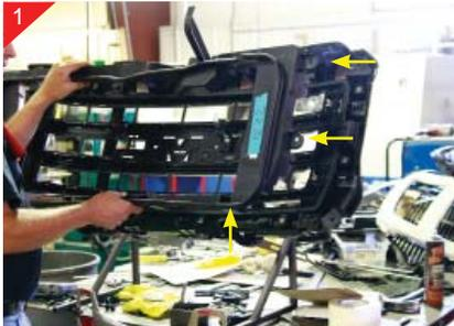
Remove stock grille shell from vehicle and lay face down on a protective work surface. Next remove the (6) 10mm bolts holding the black plastic that meet up to core support area as shown above.
