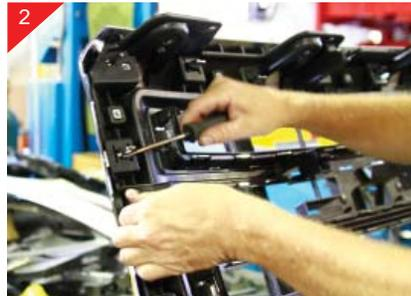
Next you will separate the black plastic from the chrome face of the shell. Do so by releasing or unclipping using a regular screwdriver to aid in releasing the (18) clips.
